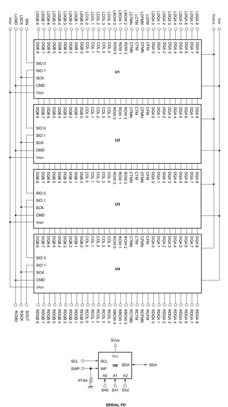
**Remarks** 1. Rambus Channel signals form a loop through the RIMM module, with the exception of the SIO chain.
