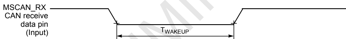
Figure 10-14 Bus Wake-up Detection
