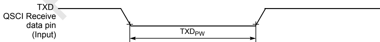
Figure 10-13 TXD Pulse Width
