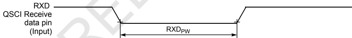
Figure 10-12 RXD Pulse Width
