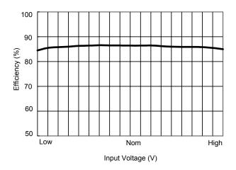
Efficiency vs Input Voltage ( Dual Output )
