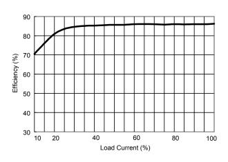
Efficiency vs Output Load (Dual Output)
