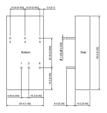
**Tolerance** Millimeters Inches .XX±0.01 .X±0.25 .XXX±0.01 .XX±0.25 Pin ±0.05 ±0.002
