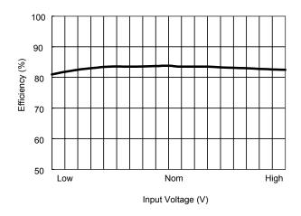
Efficiency vs Input Voltage (Single Output)
