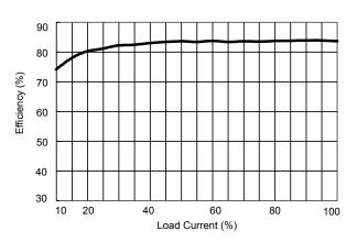
Efficiency vs Output Load (Single Output)
