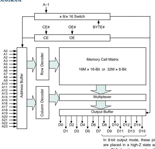
In 8-bit output mode, these pins are placed in a high-Z state and pin D15 functions as the A-1 address pin.
