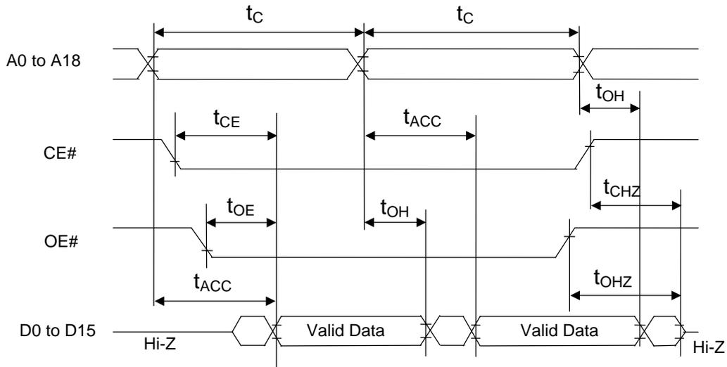
**8-Bit Read Mode (BYTE# = V<sub>IL</sub>)**
