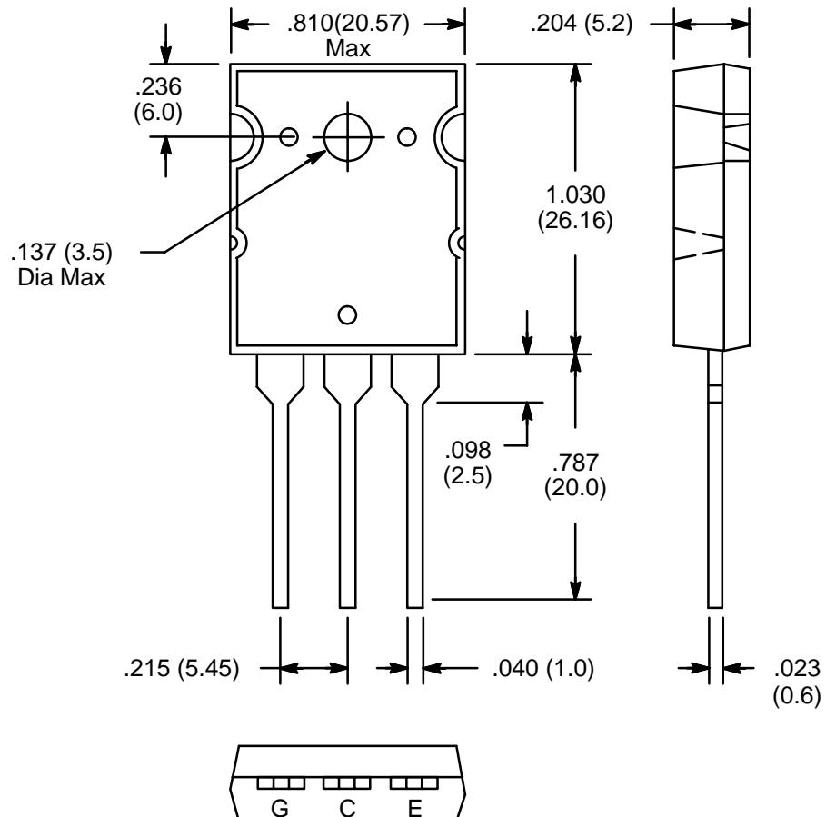
**Note:** Collector connected to heat sink.
