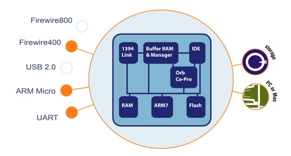
**The Oxford 911** plus is the latest generation 1394A to ATA7/ATAPI (IDE) bridge. It supports all PIO, DMA and UDMA modes up to UDMA6, delivering a sustained data transfer performance of over 40MBytes/sec. Hardware features include SBP2.0 acceleration with 'fast start', in addition to dual disk striping and transparent spanning capabilities, all designed to achieve maximum data throughput.
