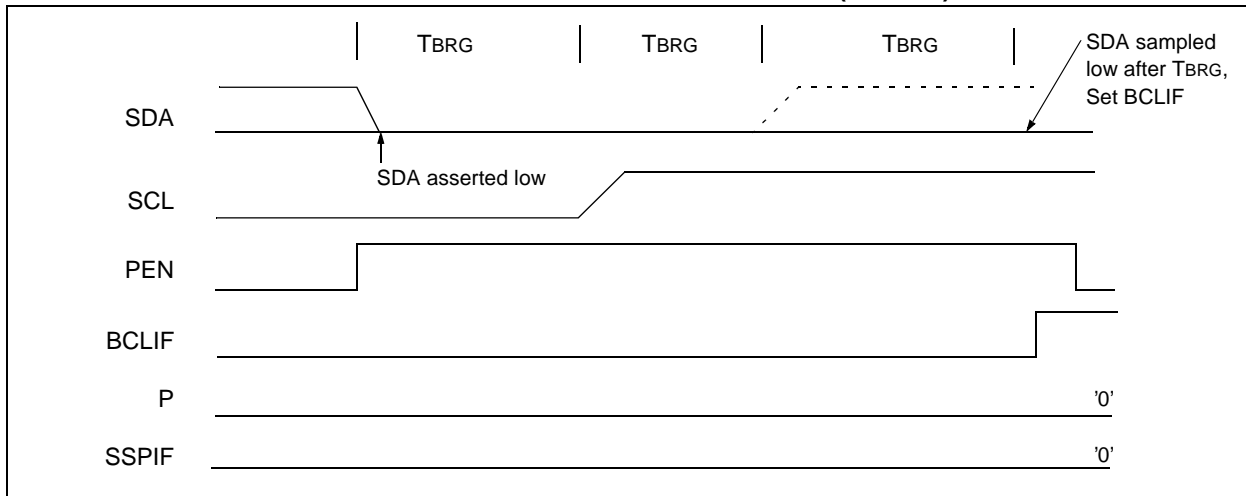
FIGURE 14-29: BUS COLLISION DURING A STOP CONDITION (CASE 1)
