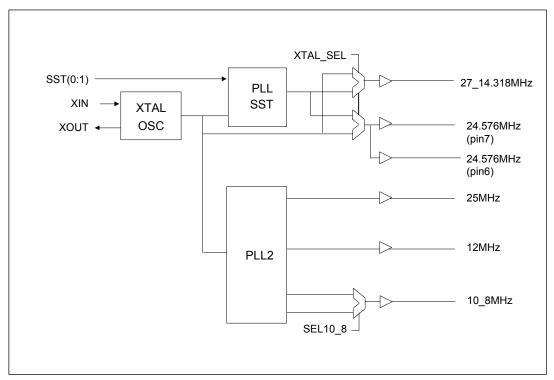
Note 1: In order to use VDD25M as power source for 10\_8MHz (pin 13), 24.576MHz (pin 7), and 12MHz (pin 12), it is necessary to select this feature through the VDD\_SEL and SEL10\_8M inputs (see Power Selection and 10\_8MHz Frequency Selection Tables on p.1).
