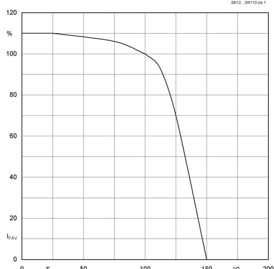
Fig. 2 Rated forward current vs. temp. of the terminals
