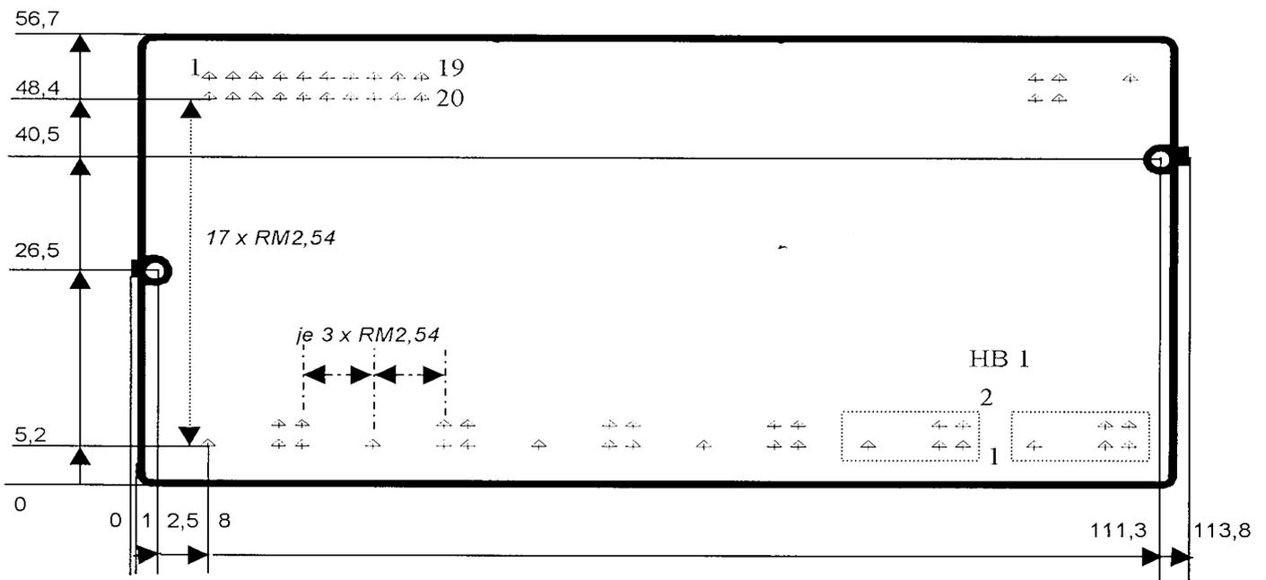
Fig. 9 Dimensional drawing, layout
