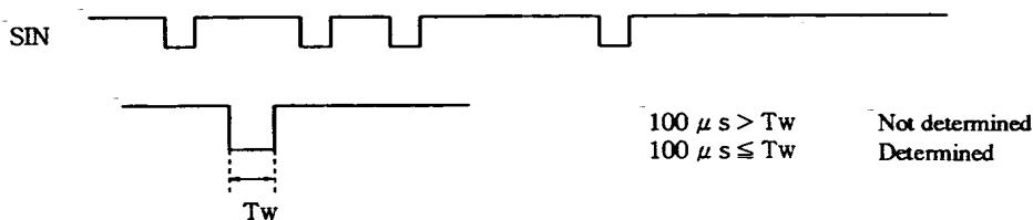
The pulse is not judged correctly unless its width Tw is 100  $\mu$ s or longer. (When Tw is from 50 to 100  $\mu$ s, the pulse may or may not be determined due to the relation with the internal clock positions.)
