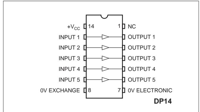
Figure 1: Pin connections (viewed from underside)
