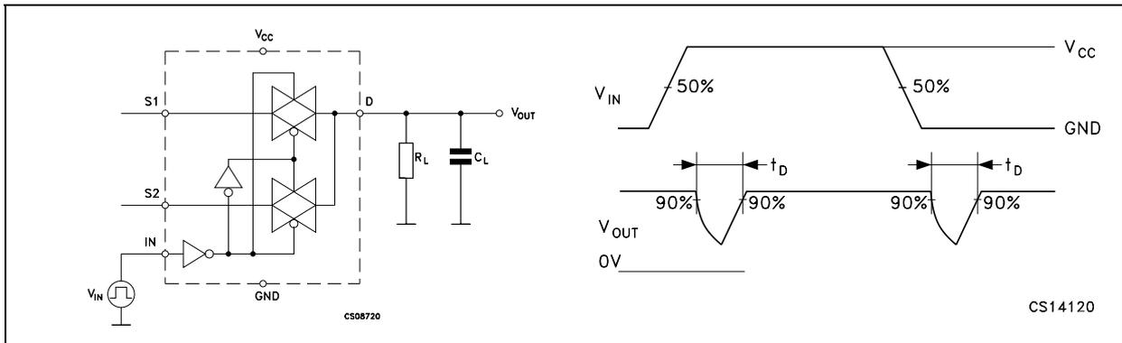
SWITCHING TIME AND CHARGE INJECTION ( $V_{GEN}=0V$ ,  $R_{GEN}=0\Omega$ ,  $R_L=1M\Omega$ ,  $C_L=100\text{pF}$ ) TURN ON,
