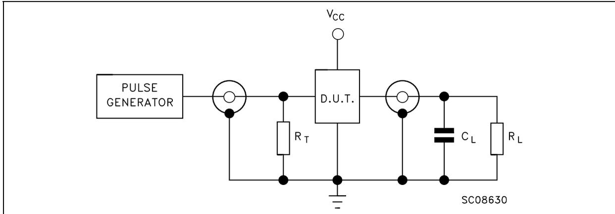
$C_L = 5/35\text{pF}$  or equivalent (includes jig and probe capacitance)
