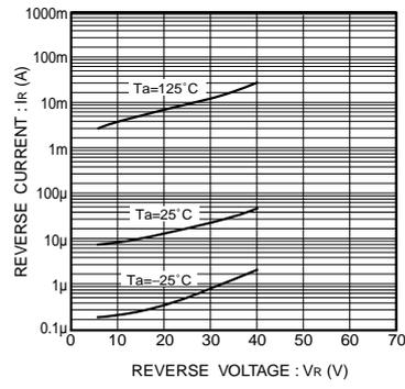
Fig.9 Reverse characteristics
