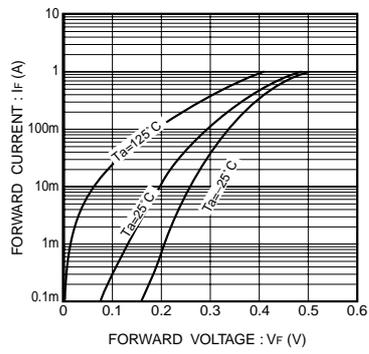
Fig.8 Forward characteristics
