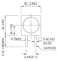
RECOMMENDED PCB LAYOUT ø0.889-2 2.54(0.1)
