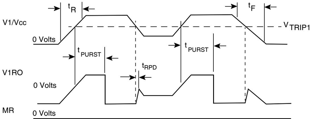
Figure 26. Manual Reset Timing Diagram
