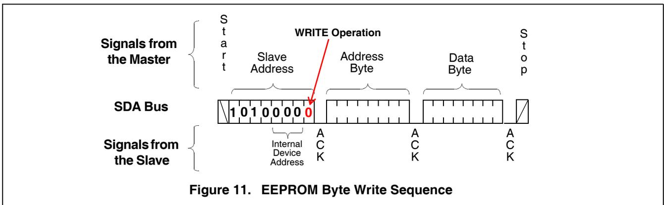
Figure 11. EEPROM Byte Write Sequence
