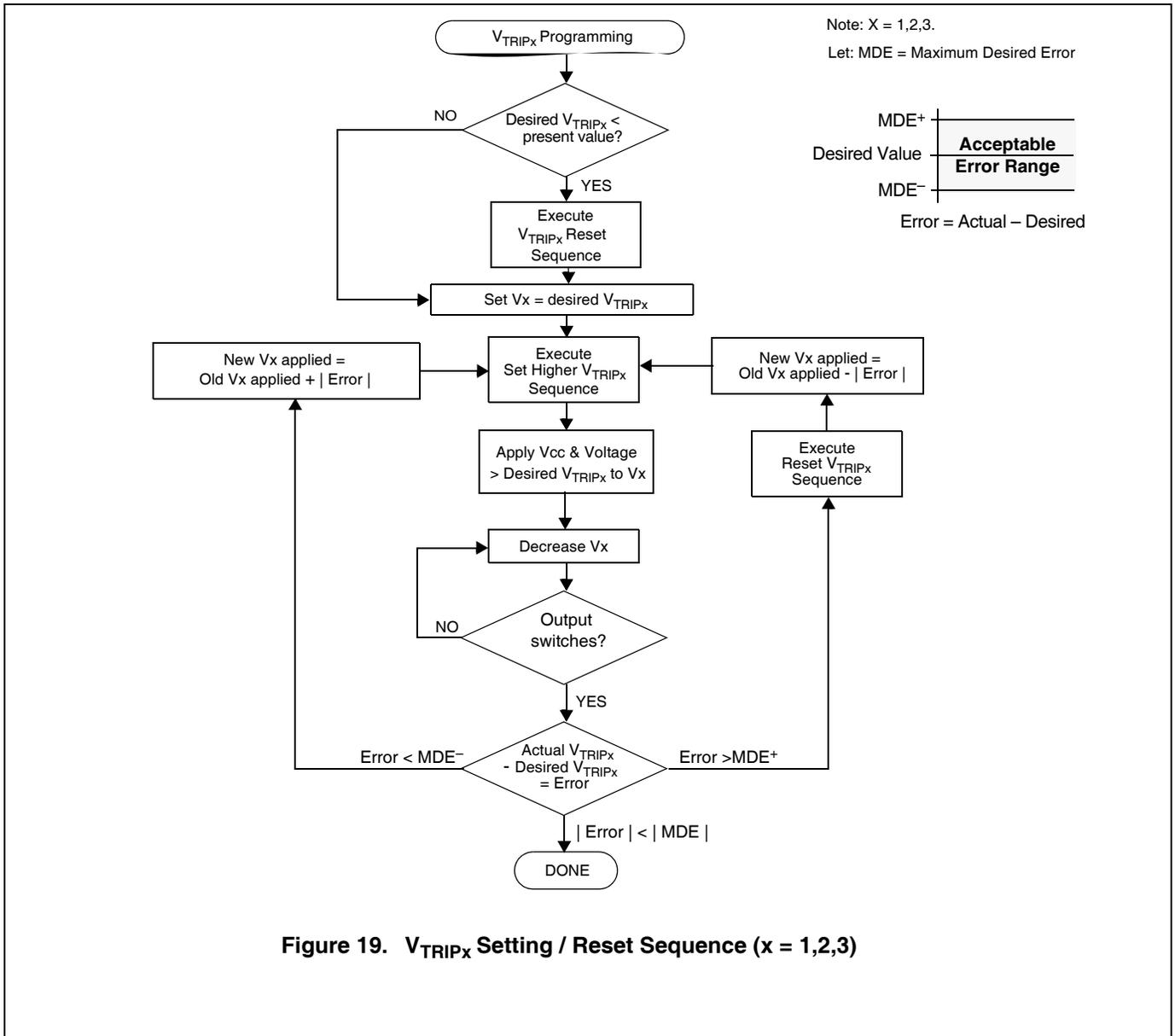
Figure 19.  $V_{TRIPx}$  Setting / Reset Sequence (x = 1,2,3)
