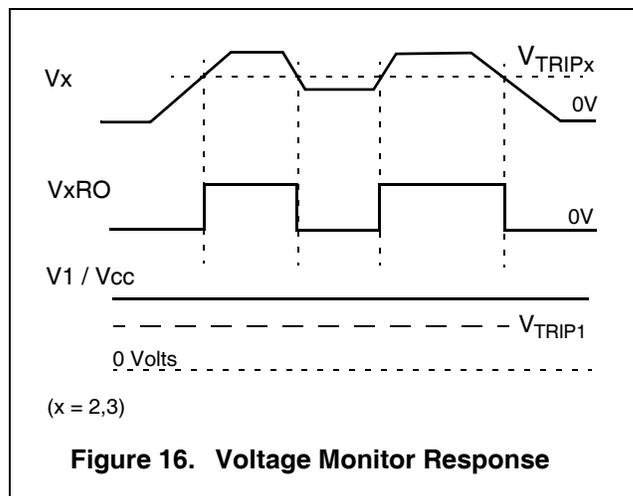
It is recommended to stop communication to the device while V1RO is HIGH. Also, setting the Manual Reset (MR) pin HIGH overrides the Power-on/Low Voltage circuitry and forces the V1RO output pin HIGH (See “Manual Reset”).
