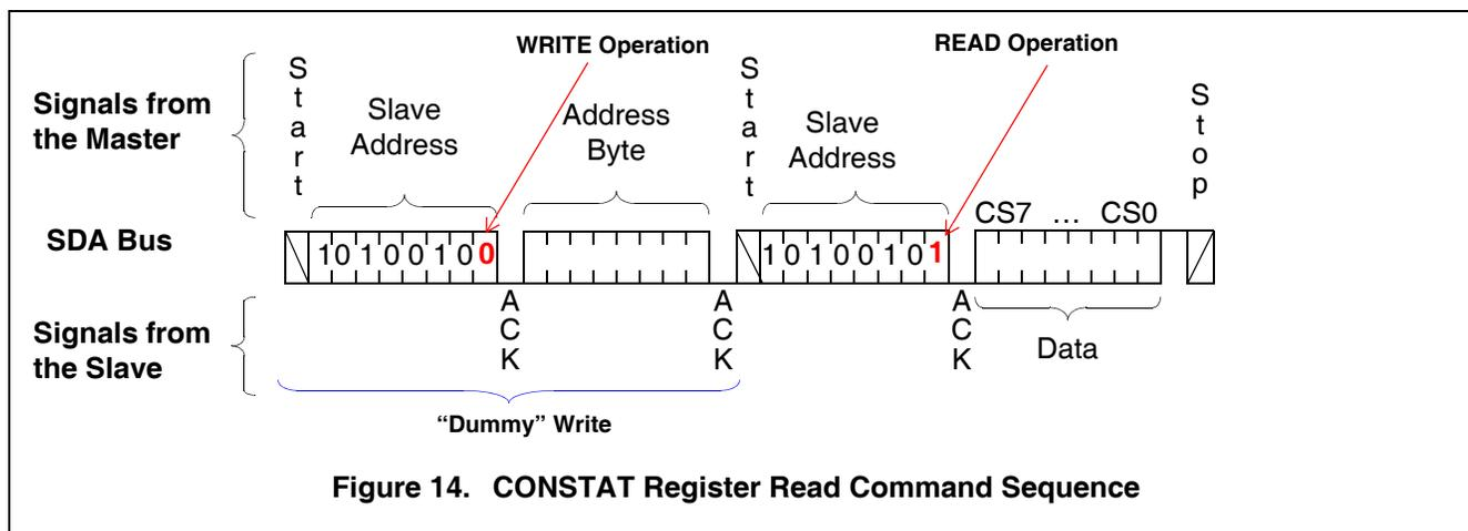
Figure 14. CONSTAT Register Read Command Sequence
