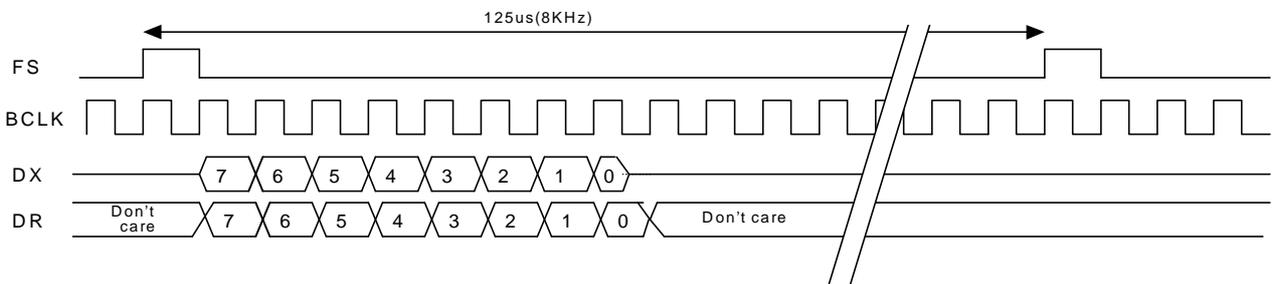
**Notice** FS must be 8kHz clock that is synchronized with BCLK.
