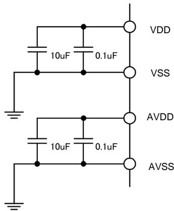
Please adjust capacitors in response to the noise environment on the power source.
