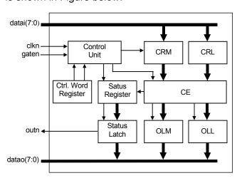
The central element of each Counter is **CE** module - Counting Element - 16 bit pre-
