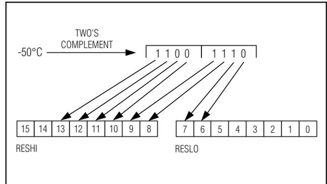
Figure 2. Conversion of Temperature Done in Two's Complement
