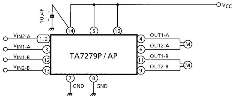
Problems may result if a capacitor is inserted in parallel to the motor.
