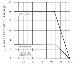
$T_{C}$ , CASE TEMPERATURE ( $\Box$ C) Fig. 1 Forward Current Derating Curve
