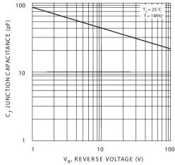
Fig. 4 Typical Junction Capacitance
