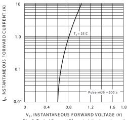
Fig. 2 Typical Forward Characteristics (per element)
