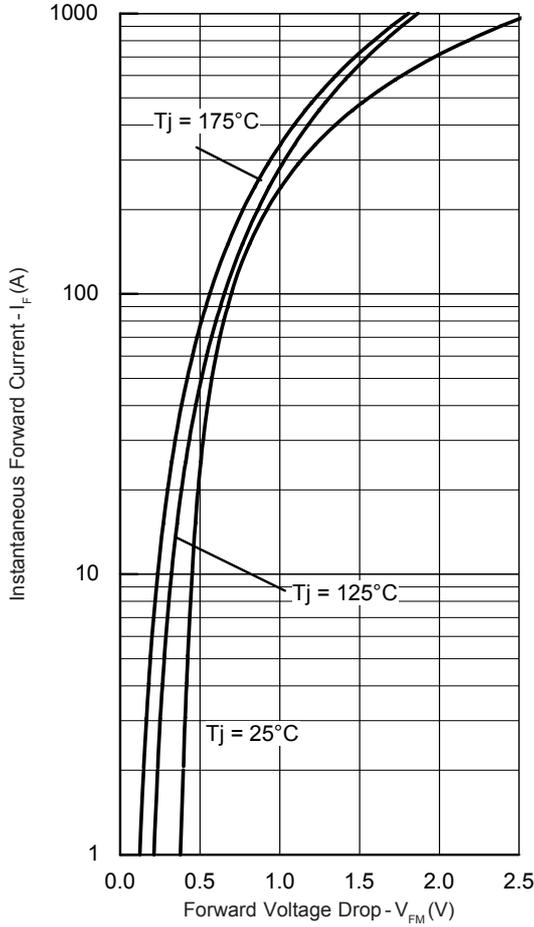
Fig. 1 - Max. Forward Voltage Drop Characteristics
