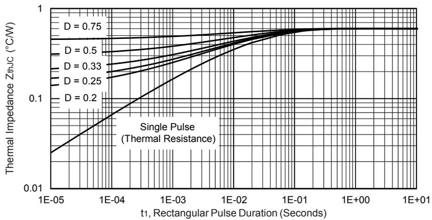
Fig. 4 - Max. Thermal Impedance  $Z_{thJC}$  Characteristics
