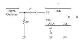
1Vp-p, 10MHz sine wave input signal
