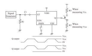
1Vp-p, 10MHz sine wave input signal
