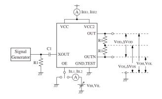
500mVp-p, sine wave C1:  $0.01\mu\text{F}$  R1:  $49.9\Omega$  Note. Connect  $0.01\mu\text{F}$  and approximately  $10\mu\text{F}$  bypass capacitors between supply (V<sub>CC</sub>, V<sub>CC2</sub>) and GND. Note that the  $0.01\mu\text{F}$  capacitor should have circuit wiring as short as possible.
