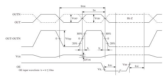
$$\begin{split} DUTY = 100 t_W / t_{PER} \ (\%) \ @ \ crossing \ point \\ \Delta V_{OD} = |V_{OD}' - V_{OD}| \end{split}$$
