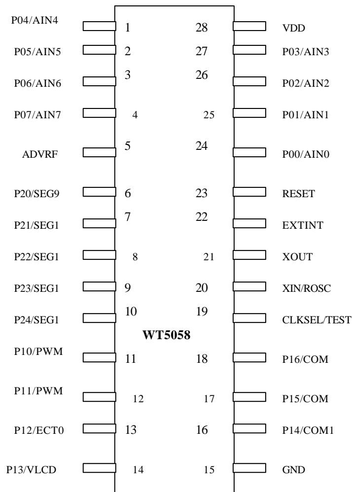
**PACKAGE PIN ASSIGNMENT (28-PIN DIP or 28-PIN SKINNY; Option #2)**
