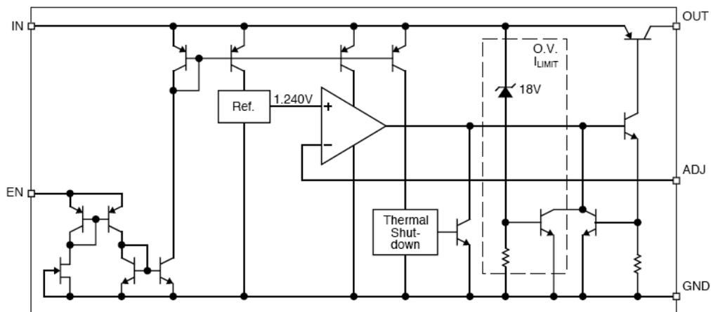
**TS39152 Adjustable Regulator Block Diagram**
