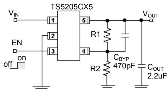
Adjustable Version:  $V_{OUT} = 1.24 (R1+R2)/R1$
