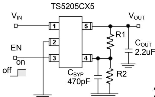
Adjustable Version:  $V_{OUT} = 1.24 (R1+R2)/R1$
