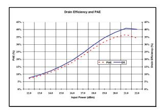
NOTE: Typical power and efficiency is shown above. The devices were biased nominally at  $V_{DS}$  = 5V,  $I_{DS}$  = 50% of  $I_{DSS}$ , at a test frequency of 1.85 GHz. The test devices were tuned (input and output tuning) for maximum output power at 1dB gain compression.
