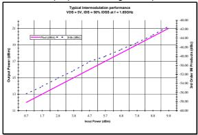
Note: pHEMT devices have enhanced intermodulation performance. This yields OIP3 values of about P1dB + 14 dB. This IMD enhancement is affected by the quiescent bias and the matching applied to the device.
