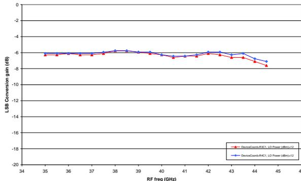
XM1000-BD: USB Conversion gain (dB) vs. RF freq (GHz)
