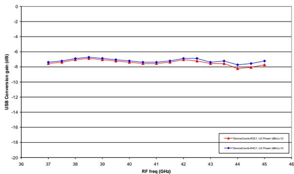
XM1000-BD: LSB Conversion gain (dB) vs. RF freq (GHz)
