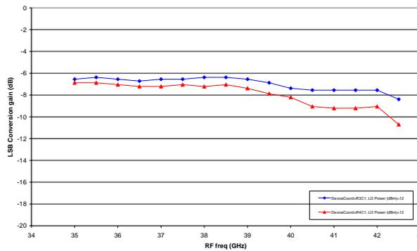
XM1000-BD: LSB Conversion gain (dB) vs. RF freq (GHz)
