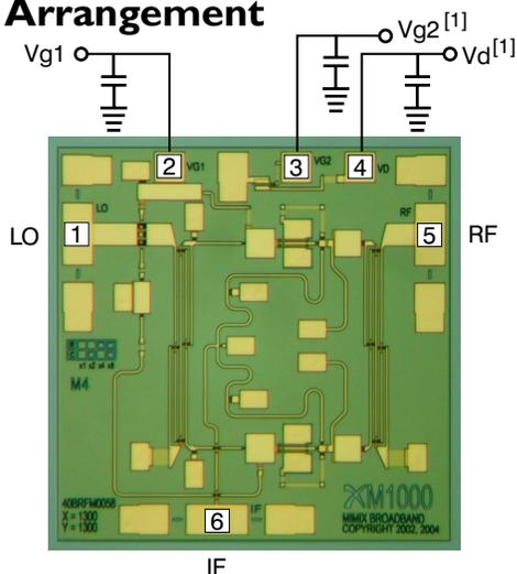
**App Note [1] Biasing** - As shown in the bonding diagram, the pHEMT mixer devices are operated using a separate gate voltage Vg1. Set Vg1=-0.6V for optimum conversion loss performance. pHEMT test device (Vd,Vg2) with 100 Ohm resistor is provided so that mixer gate bias can be corrected for local Vto.
