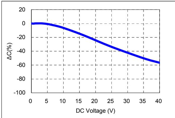
4) Bias TCC characteristics (Agilent 4284A, 1kHz, 1Vrms, 25Vdc)
