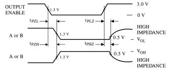
$\begin{array}{l} t_{PZL} \text{ - } S1 \text{ closed, } S2 \text{ opened} \\ t_{PZH} \text{ - } S1 \text{ opened, } S2 \text{ closed} \\ t_{PLZ}, t_{PHZ} \text{ - } S1 \text{ and } S2 \text{ closed} \end{array}$
