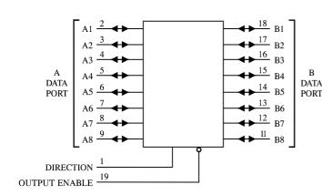
$PIN 20=V_{CC}$  PIN 10 = GND
