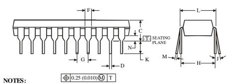
$1. \ \ \, \text{Dimensions "A", "B" do not include mold flash or protrusions.}$
