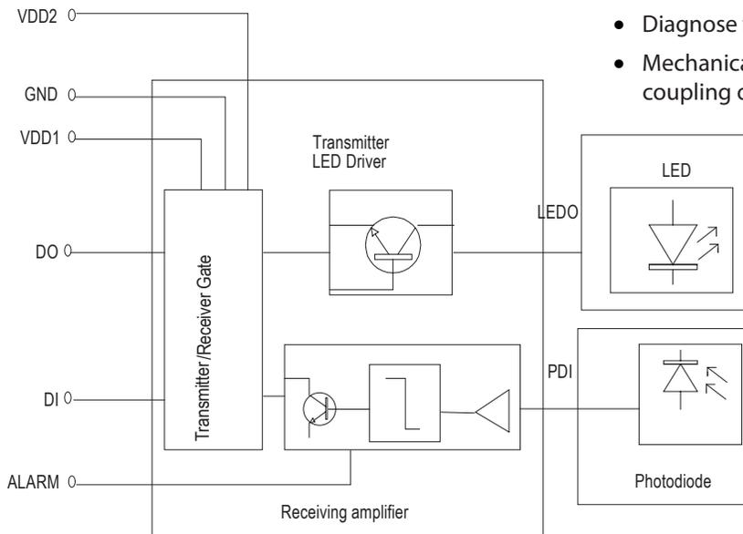
Figure 1. Basic functional units of SPF BFT3 03
