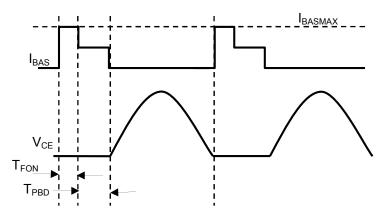
Figure 8: Base Driver Current Waveforms
