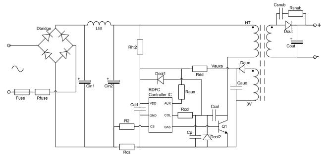
Figure 3: Typical Low Power RDFC Application Schematic
