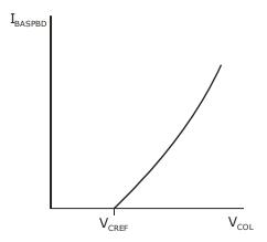
Figure 9: I<sub>BASPBD</sub> characteristic
