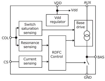
Figure 1: Block Diagram of the C2471 Controller ICs
