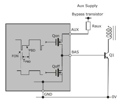
Figure 7: Primary Switch (Q1) Base Drive
