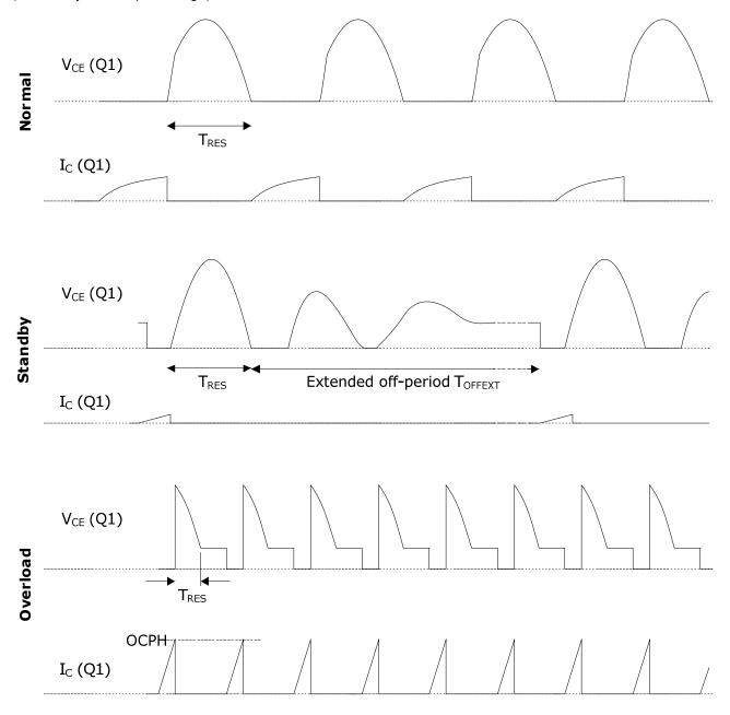
Figure 6: Typical Switch (Q1) Collector Voltage (V<sub>CE</sub>) and Current (I<sub>C</sub>) Waveforms
