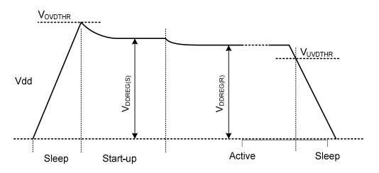
Figure 4: VDD Pin Waveform (V<sub>DD</sub>) During Initial Power-up and Power-down
