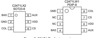
Figure 2: C2471 Pin Assignment (drawings are not to scale)
