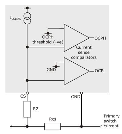
Figure 10: Current Sense Diagram
