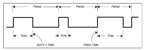
Fig. -2 PWM Output Timing Diagram
