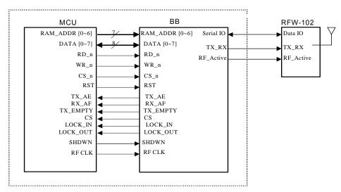
Fig. 8-1 Parallel Interface between the MCU and RFW-102 through BB
