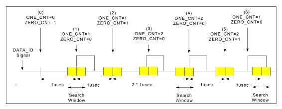
Fig. 8-4 Carrier-Sense Example
