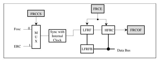
Fig. 13-2 Timer 1 Function Block Diagram
