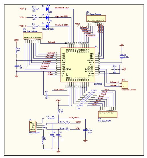
Fig. 18 USB Keyboard Circuit
