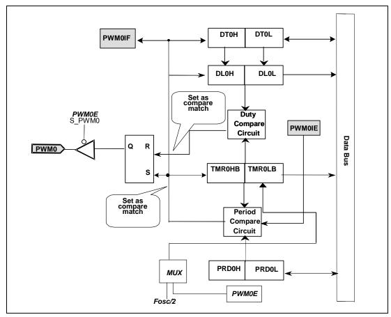
Fig. 10-1 PWM Functional Block Diagram
