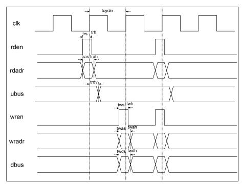
Fig. 9-2 MCU Interface Timing Diagram
