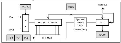
Fig. 13-1 Function Block Diagram of TCC
