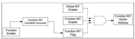
Fig. 11 Block Diagram of Interrupts
