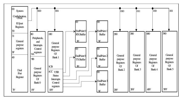
Fig. 6-2 Configuration of Data Memory (RAM) for EM77930
