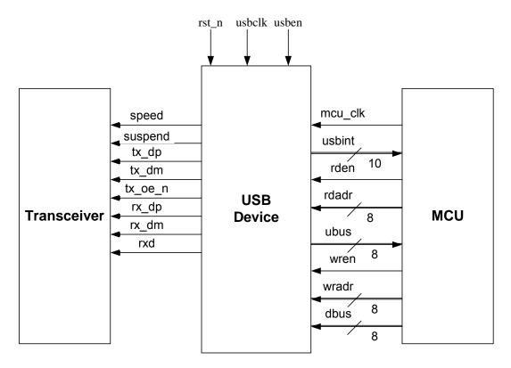
Fig. 9-1 USB Function Block Diagram of the EM77930
