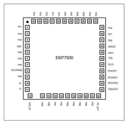
Fig. 3 Pad and Pins Configuration of EM77930
