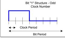
Fig. 8-3 Bit Structure of the BB output to the RFW-102
