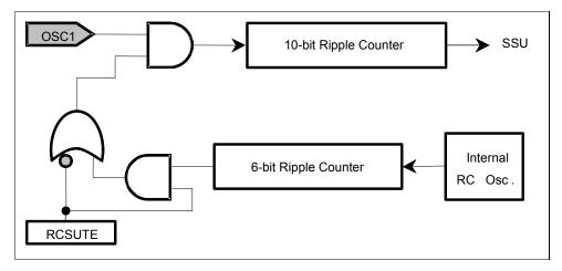
Fig. 13 System Set-up Time
