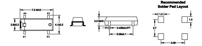
All dimensions are in millimeters. See page 31 for tape and reel specifications.
