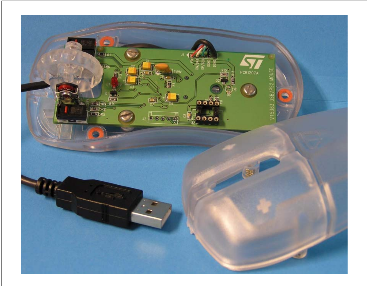
Figure 6. STV-363-R01 - USB/PS2 mouse reference design board
