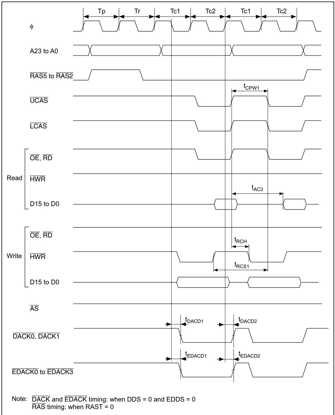
Figure 26.16 DRAM Access Timing: Two-State Burst Access
