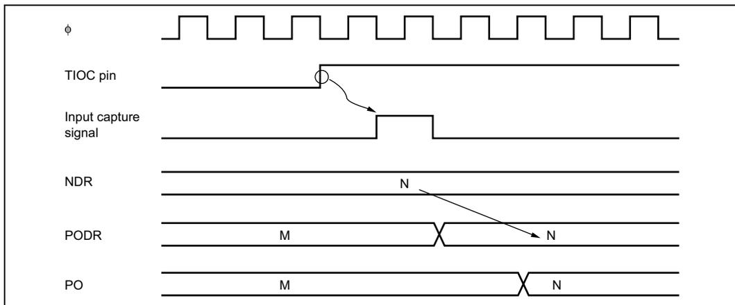
**Figure 12.11 Pulse Output Triggered by Input Capture (Example)**
