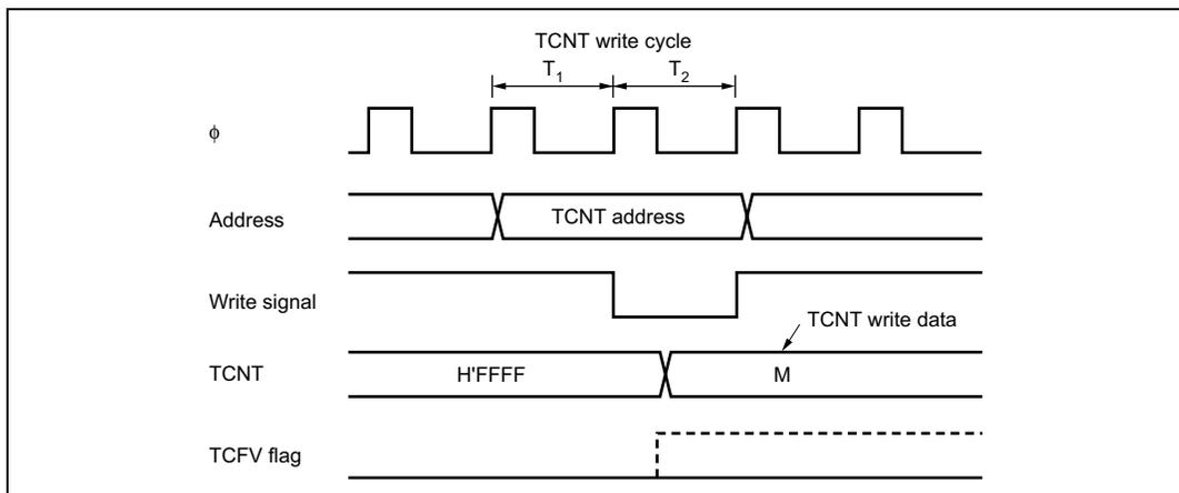
**Figure 11.53 Contention between TCNT Write and Overflow**
