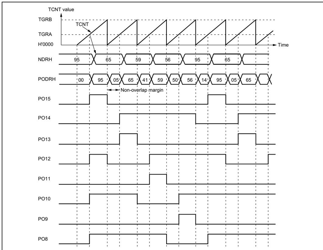
**Figure 12.9 Non-Overlapping Pulse Output Example (Four-Phase Complementary)**
