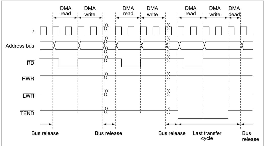
**Figure 7.18 Example of Short Address Mode Transfer**
