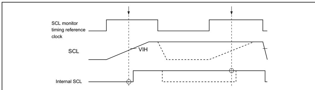
**Figure 16.18 Timing of the Bit Synchronous Circuit**
