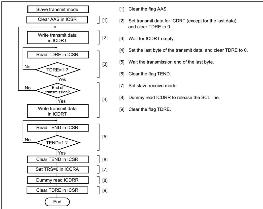
**Figure 16.16 Sample Flowchart for Slave Transmit Mode**
