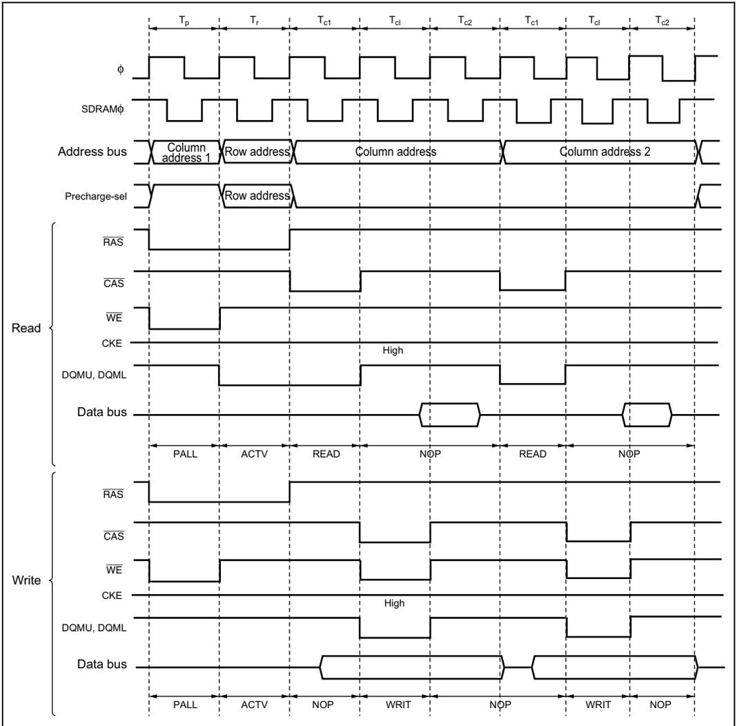
**Figure 6.52 Operation Timing of Burst Access
