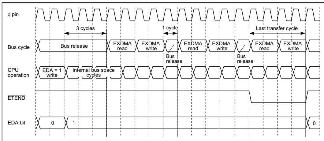
**Figure 8.28 Auto Request/Cycle Steal Mode/Normal Transfer Mode
