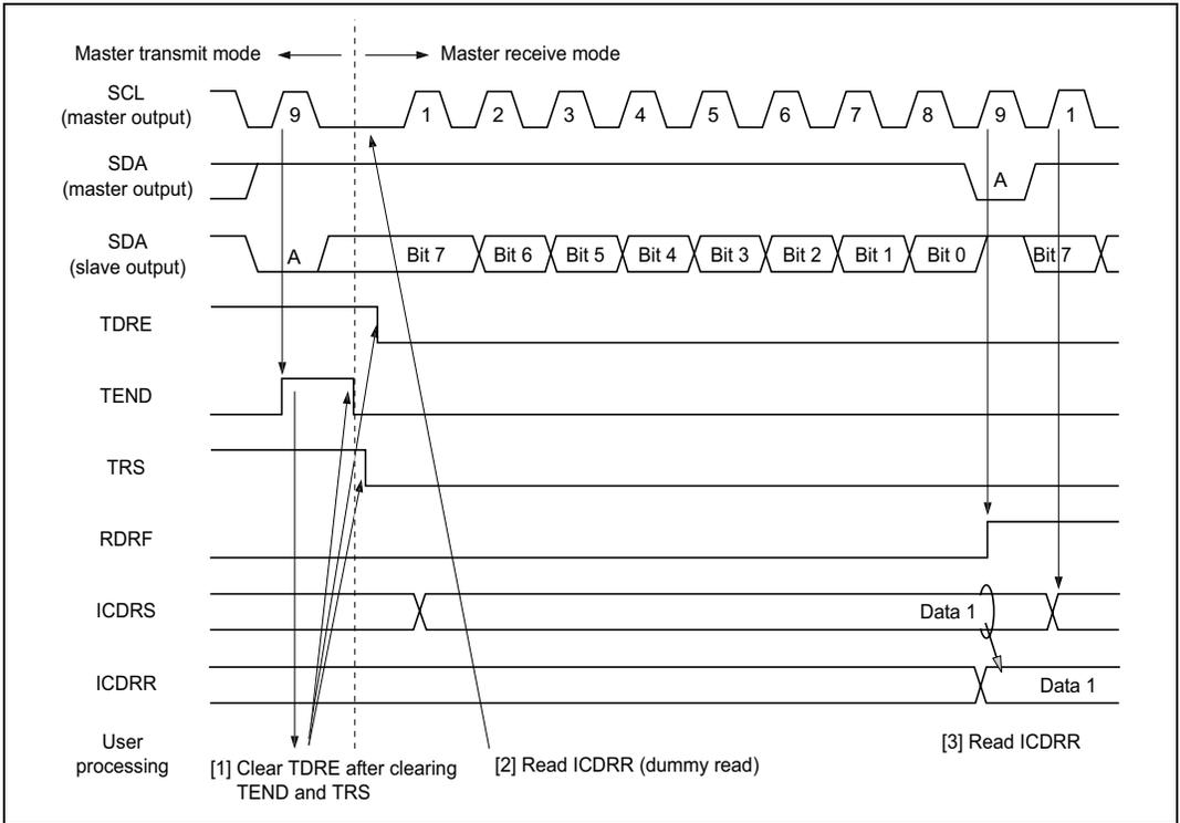
**Figure 16.7 Master Receive Mode Operation Timing 1**
