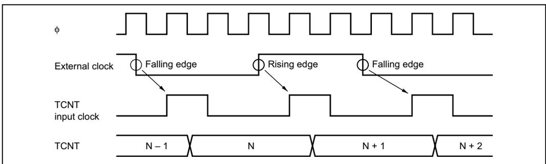
**Figure 11.31 Count Timing in External Clock Operation**
