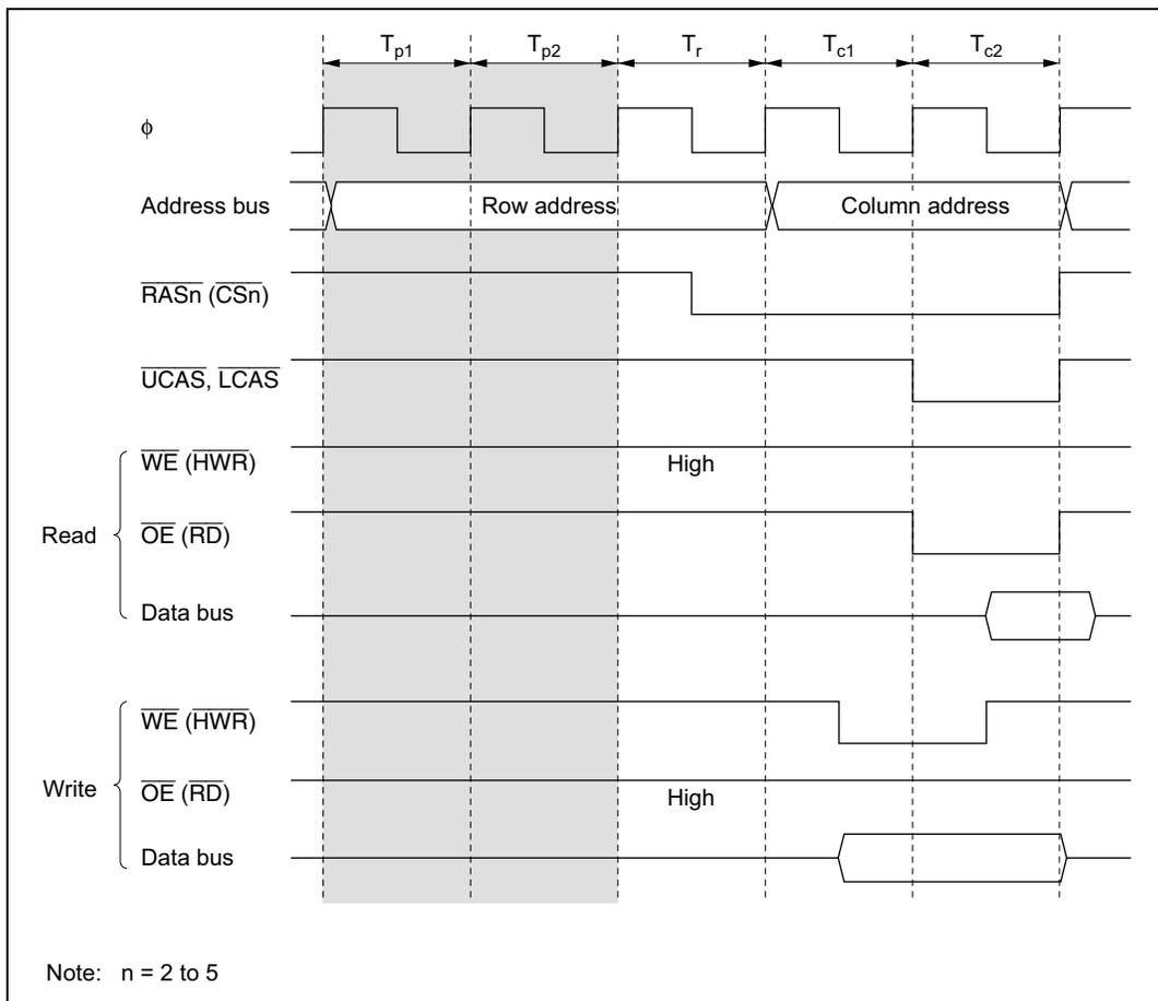
**Figure 6.25 Example of Timing with Two-State Precharge Cycle
