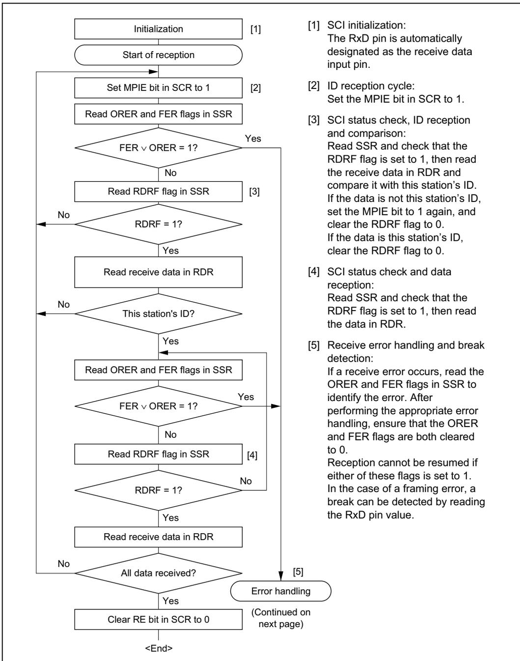
Figure 15.13 Sample Multiprocessor Serial Reception Flowchart (1)
