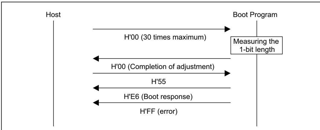
**Figure 21.18 Bit-Rate-Adjustment Sequence**
