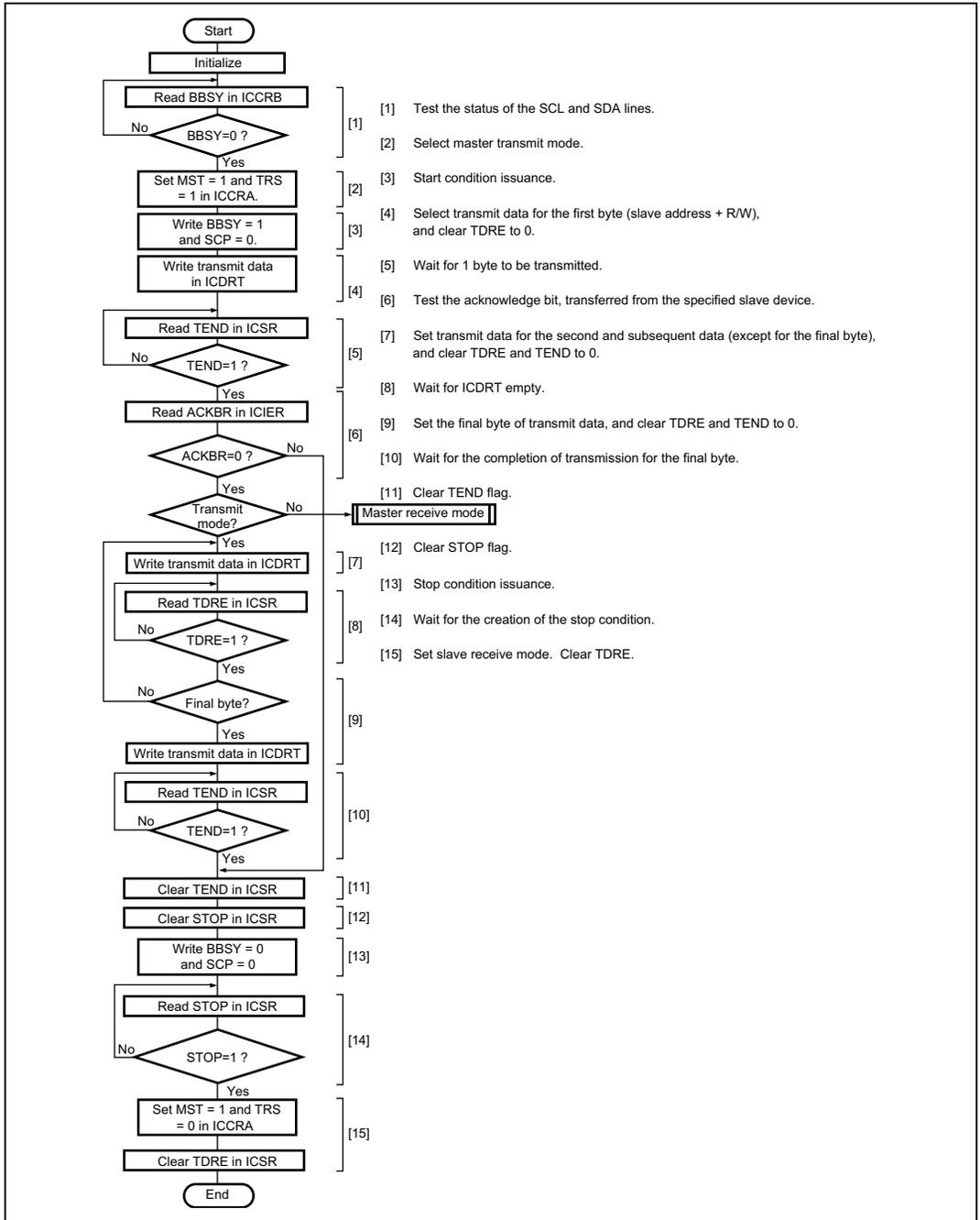
Figure 16.14 Sample Flowchart for Master Transmit Mode
