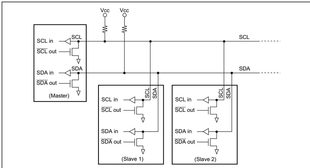
**Figure 16.2 External Circuit Connections of I/O Pins**
