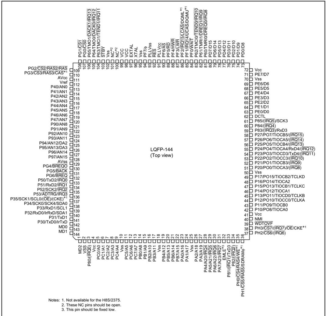
Figure 1.7 Pin Arrangement for H8S/2375 and H8S/2375R
