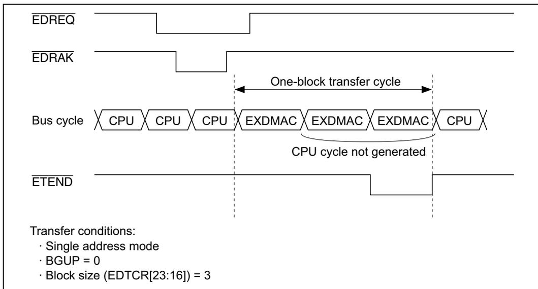
**Figure 8.8 Example of Timing in Block Transfer Mode**
