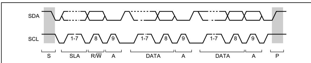
Figure 16.4 I<sup>2</sup>C Bus Timing
