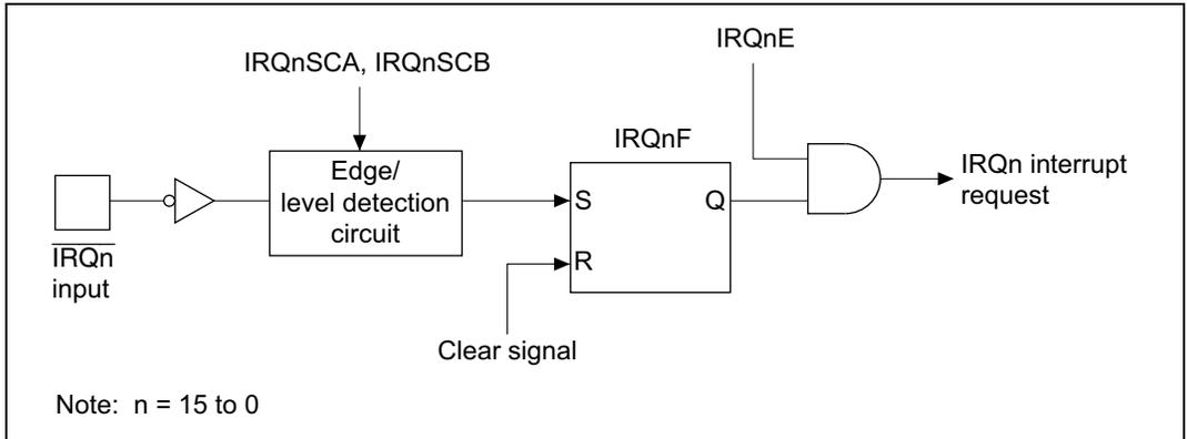
**Figure 5.2 Block Diagram of Interrupts IRQ15 to IRQ0**
