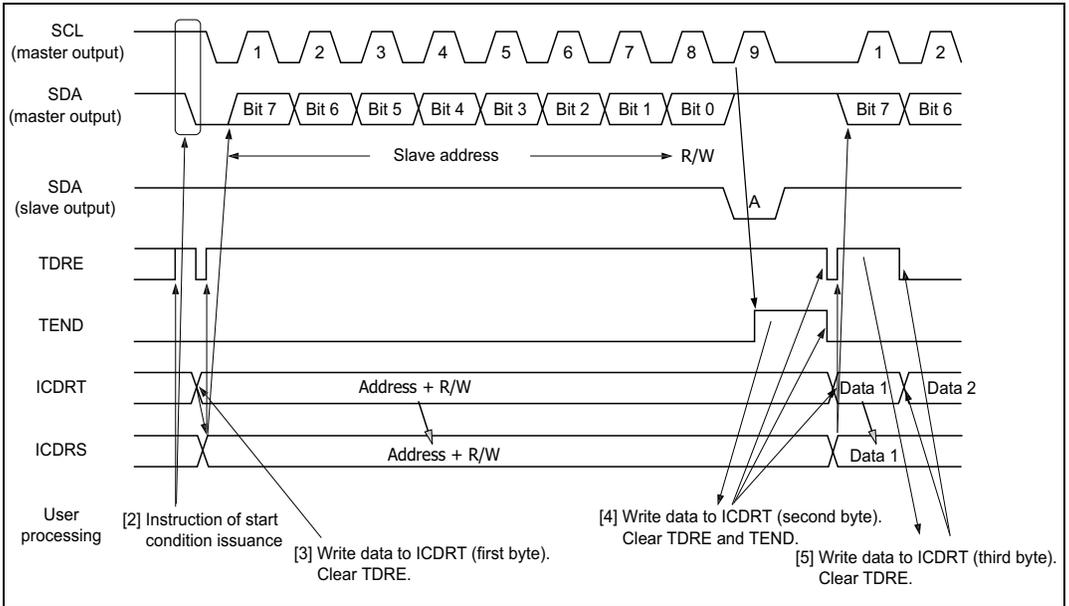
**Figure 16.5 Master Transmit Mode Operation Timing 1**
