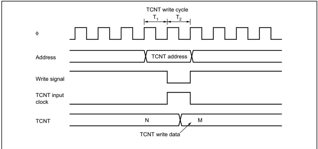
**Figure 11.46 Contention between TCNT Write and Increment Operations**
