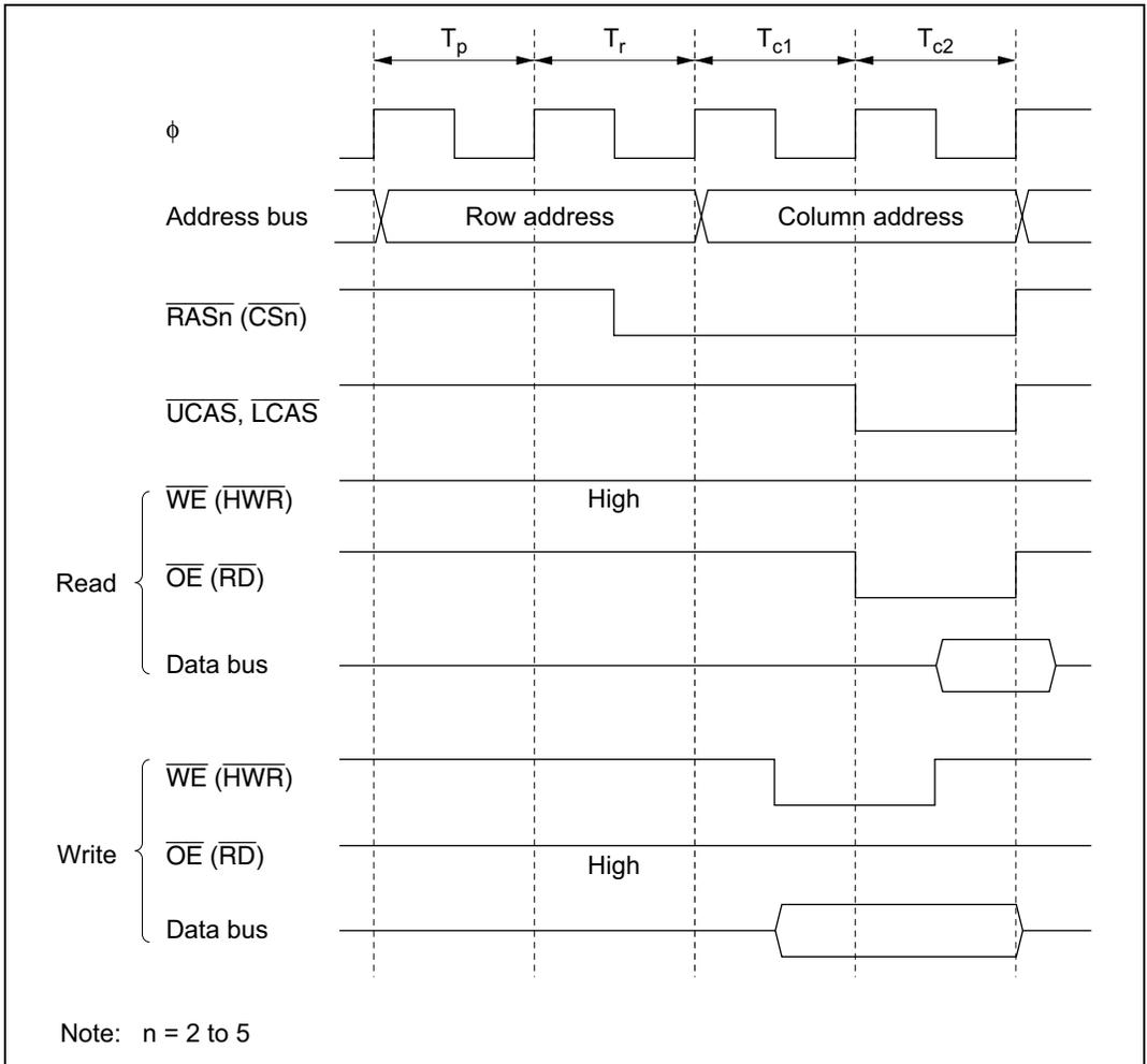
**Figure 6.21 DRAM Basic Access Timing (RAST = 0, CAST = 0)**
