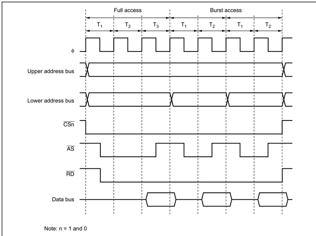
**Figure 6.63 Example of Burst ROM Access Timing
