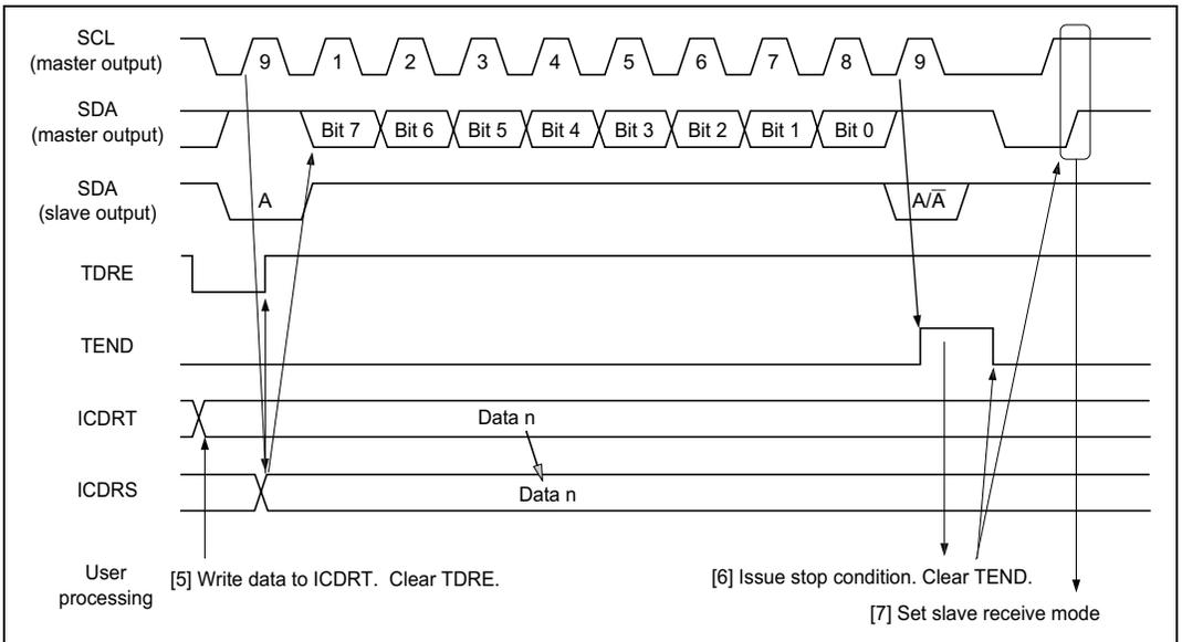
**Figure 16.6 Master Transmit Mode Operation Timing 2**
