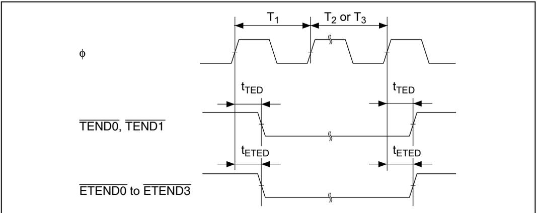
Figure 26.30 DMAC and EXDMAC  $\overline{TEND}/\overline{ETEND}$  Output Timing
