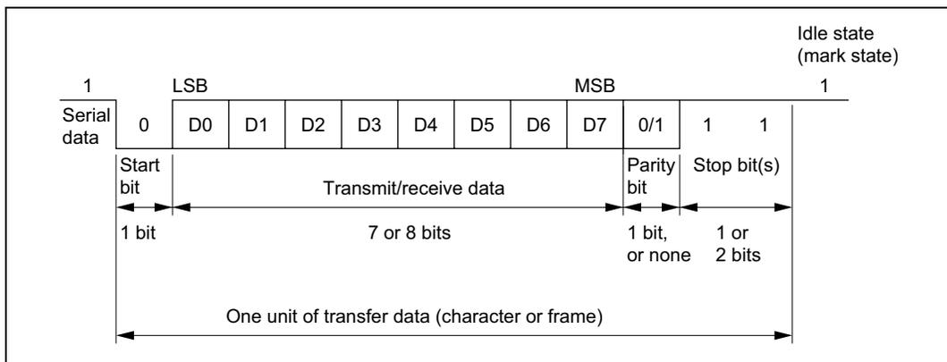
**Figure 15.2 Data Format in Asynchronous Communication
