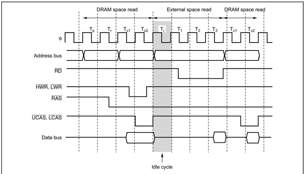
**Figure 6.78 Example of Idle Cycle Operation after DRAM Write Access
