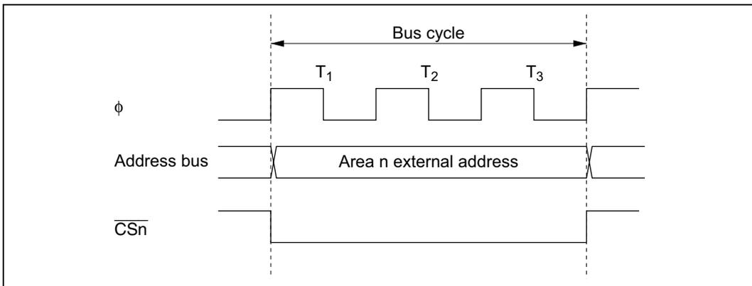
Figure 6.7  $\overline{CSn}$  Signal Output Timing (n = 0 to 7)
