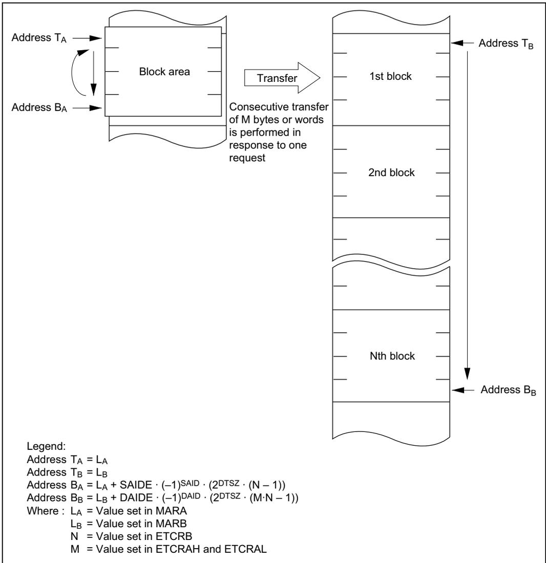
**Figure 7.14 Operation in Block Transfer Mode (BLKDIR = 1)**
