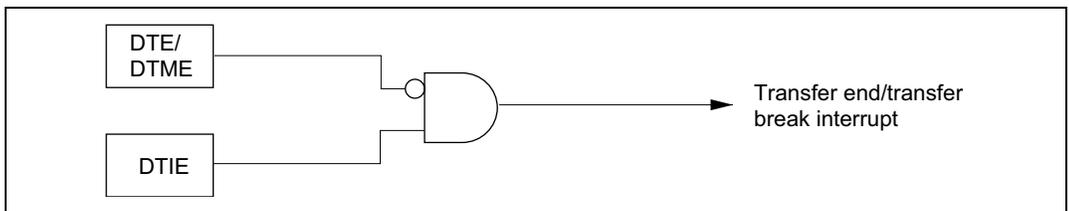
**Figure 7.38 Block Diagram of Transfer End/Transfer Break Interrupt**
