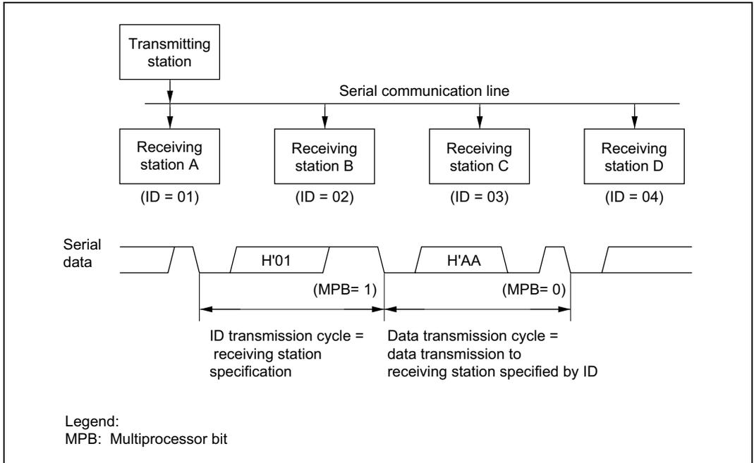
**Figure 15.10 Example of Communication Using Multiprocessor Format
