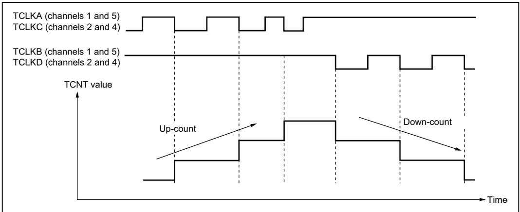
Figure 11.27 Example of Phase Counting Mode 3 Operation
