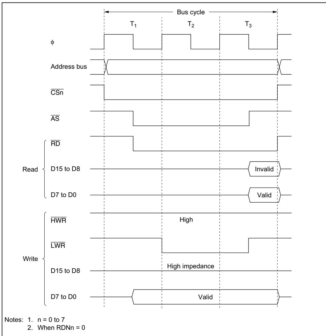
**Figure 6.16 Bus Timing for 16-Bit, 3-State Access Space
