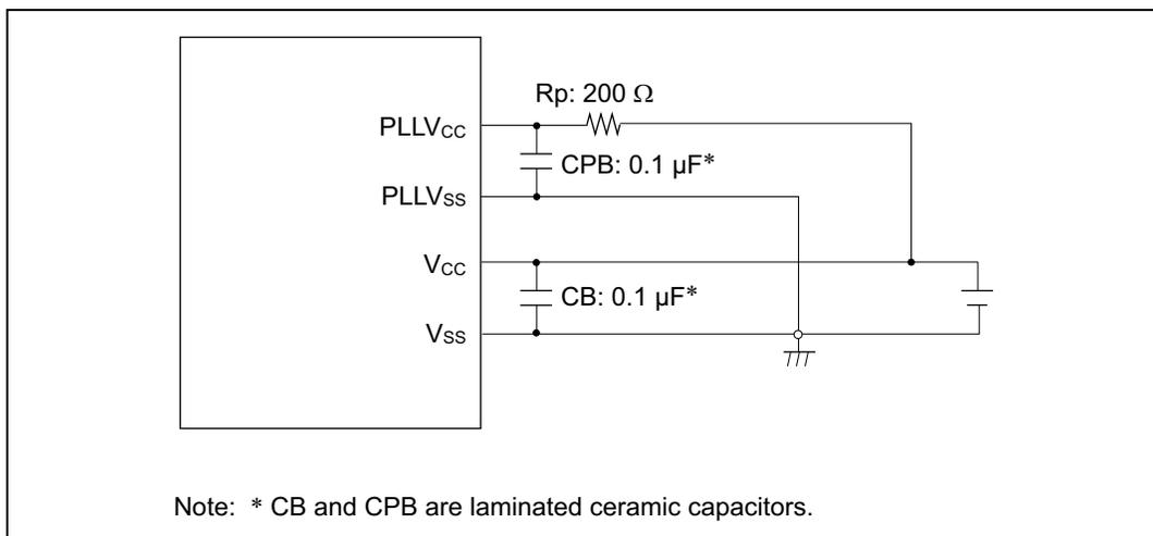
**Figure 23.7 Recommended External Circuitry for PLL Circuit**
