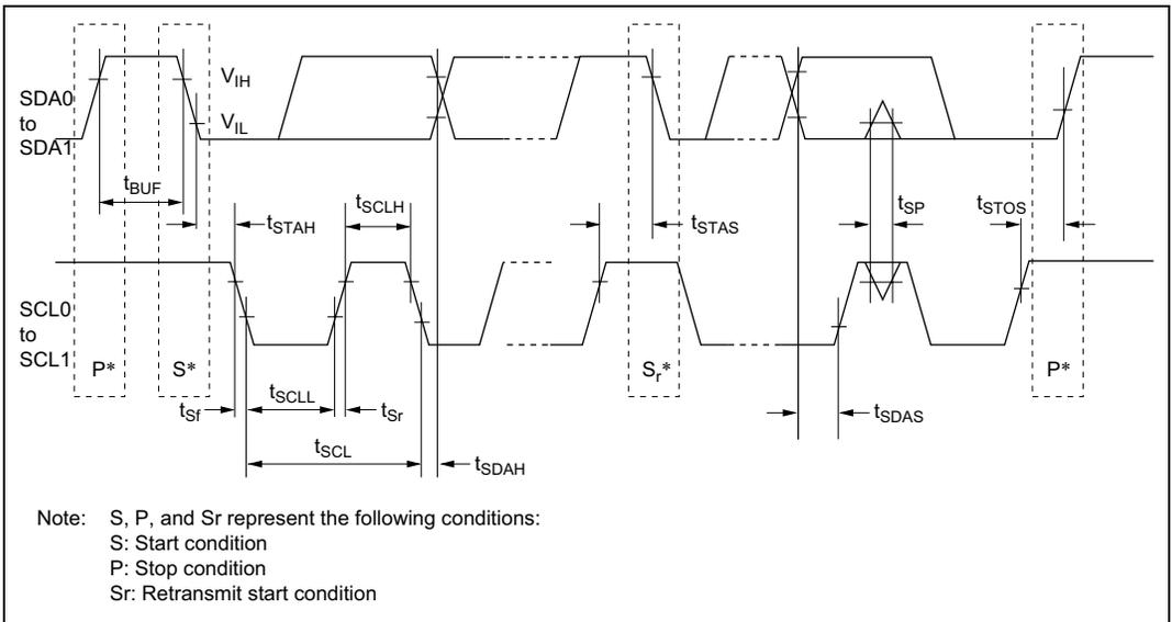
**Figure 26.44 I<sup>2</sup>C Bus Interface 2 Input/Output Timing (Option)**
