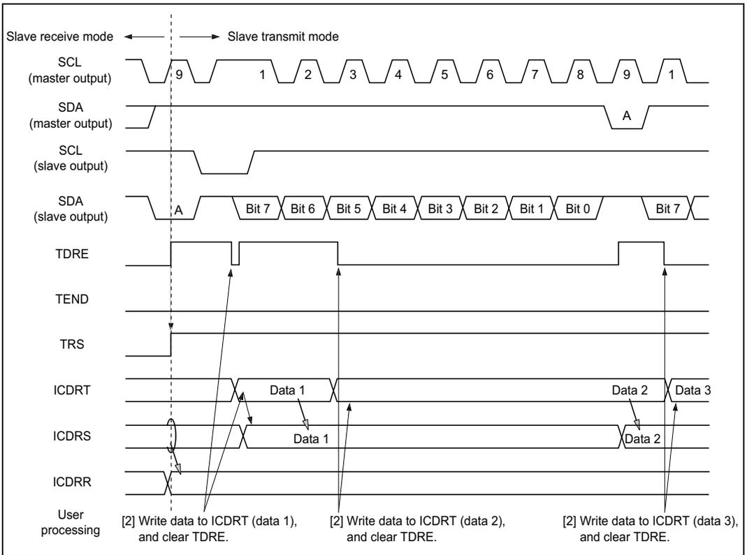
**Figure 16.9 Slave Transmit Mode Operation Timing 1**
