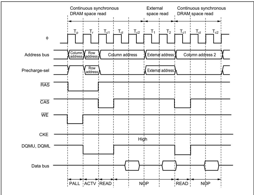
**Figure 6.53 Example of Operation Timing in RAS Down Mode
