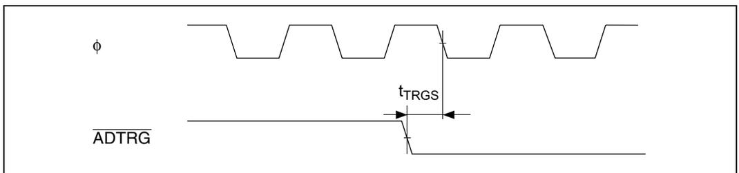
Figure 26.43 A/D Converter External Trigger Input Timing
