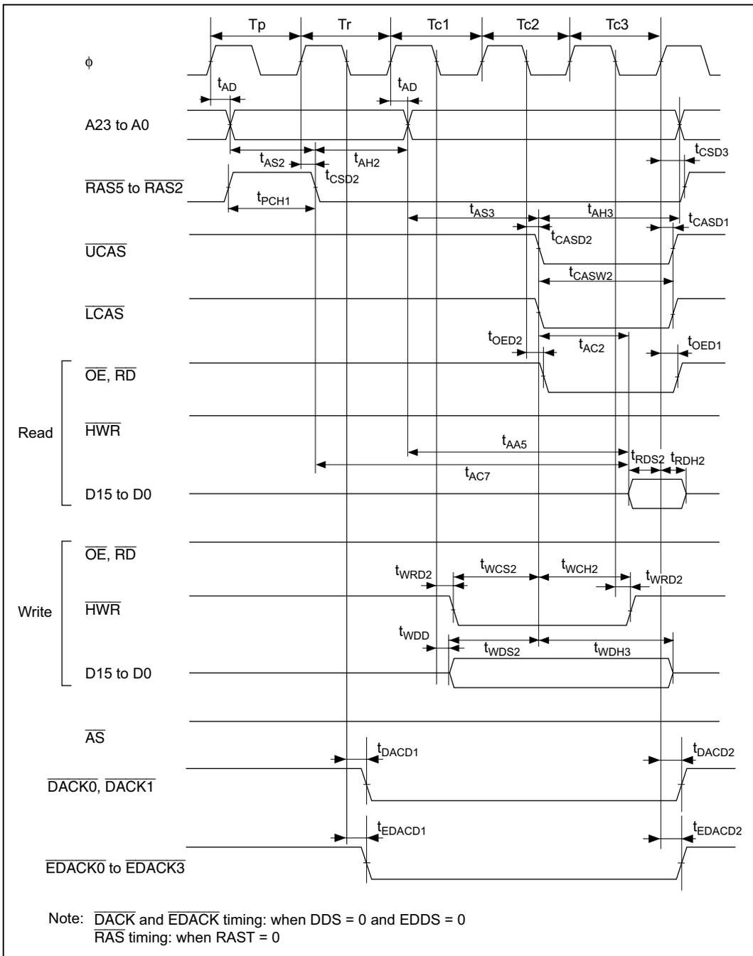
Figure 26.17 DRAM Access Timing: Three-State Access (RAST = 1)
