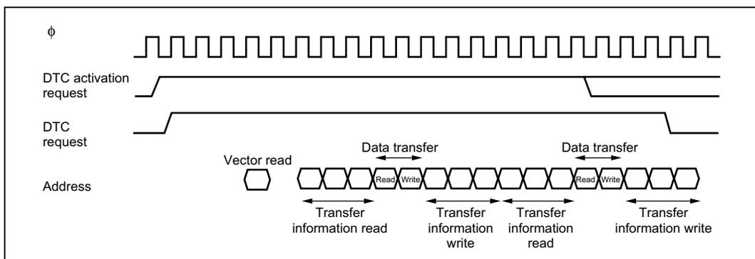
**Figure 9.12 DTC Operation Timing (Example of Chain Transfer)**
