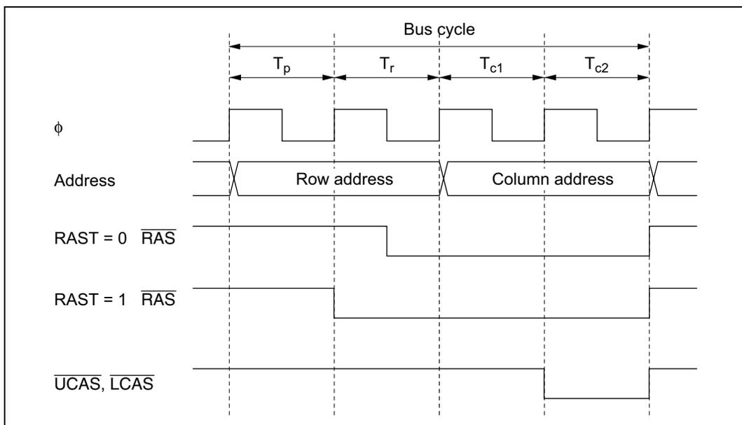
**Figure 6.4**  $\overline{\text{RAS}}$  Signal Assertion Timing
