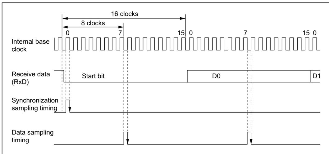
Figure 15.3 Receive Data Sampling Timing in Asynchronous Mode
