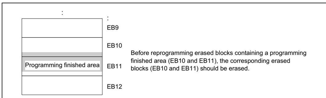
— When the erasure preparation notice is received, the state for waiting erase-block data is entered. The erase-block number must be transmitted following the erasing command. When the erasure is finished, the erase-block number must be set to H'FF and transmitted. Then the state for waiting erase-block data is returned to the state for waiting
