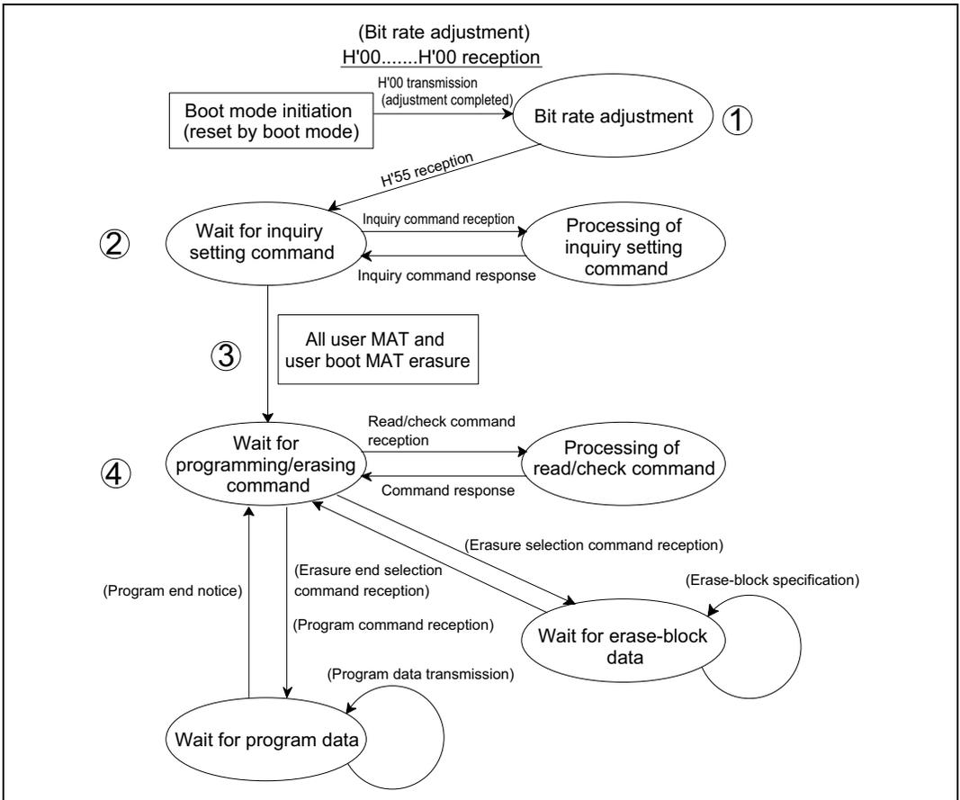
Figure 21.8 Overview of Boot Mode State Transition Diagram
