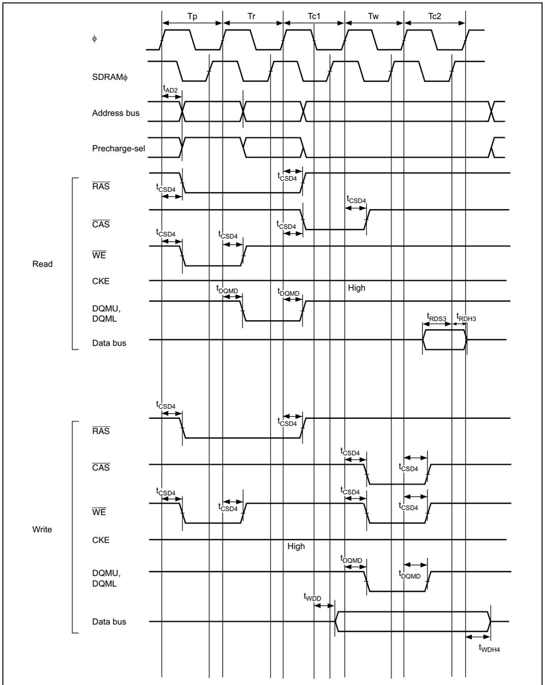
Figure 26.25 Synchronous DRAM Basic Access Timing (CAS Latency 2)
