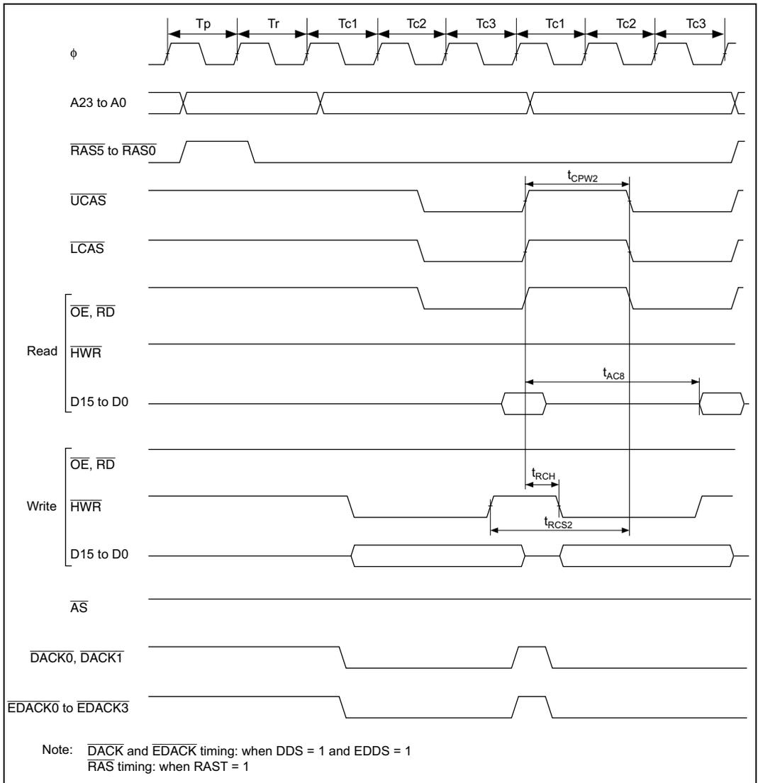
Figure 26.18 DRAM Access Timing: Three-State Burst Access
