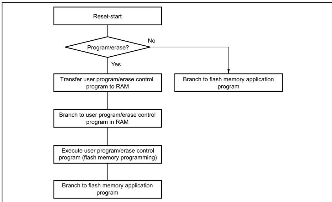
**Figure 20.6 Programming/Erasing Flowchart Example in User Program Mode**
