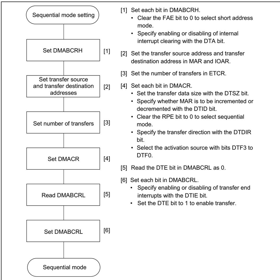
**Figure 7.4 Example of Sequential Mode Setting Procedure**
