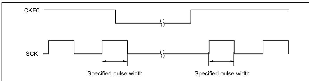
**Figure 15.31 Timing for Fixing Clock Output Level**
