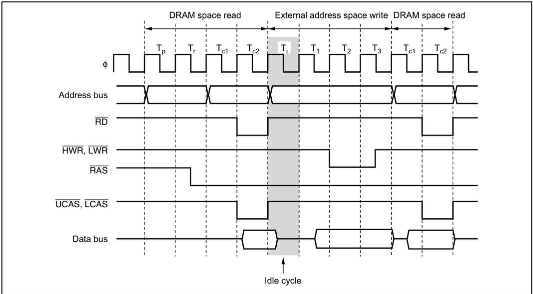
**Figure 6.77 Example of Idle Cycle Operation after DRAM Access
