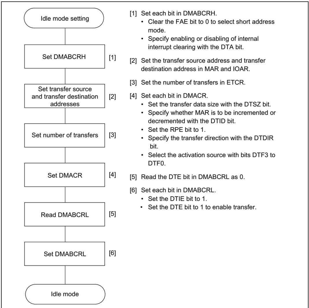
**Figure 7.6 Example of Idle Mode Setting Procedure**
