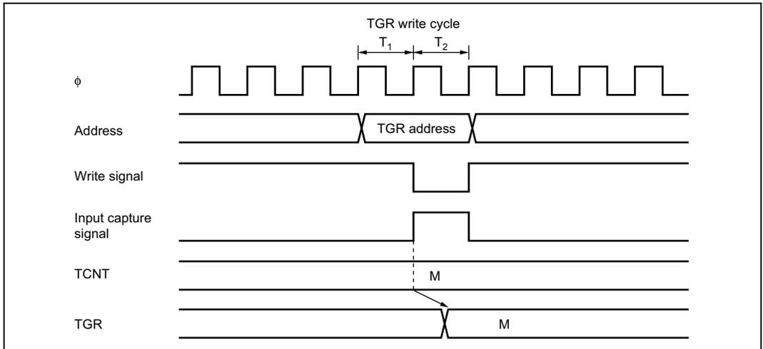
**Figure 11.50 Contention between TGR Write and Input Capture**
