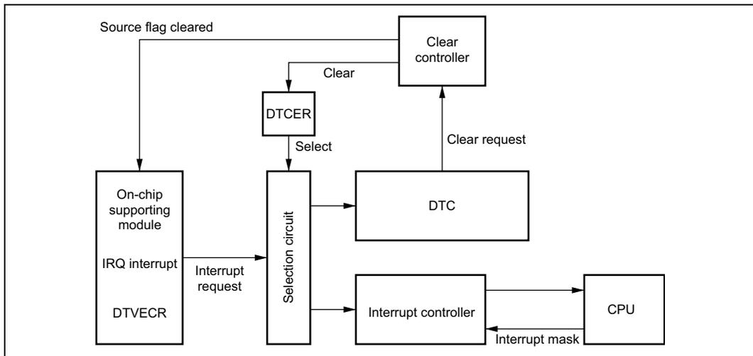
**Figure 9.2 Block Diagram of DTC Activation Source Control**
