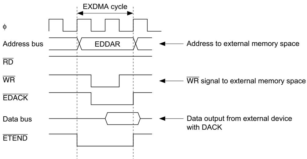
Figure 8.4 Example of Timing in Single Address Mode
