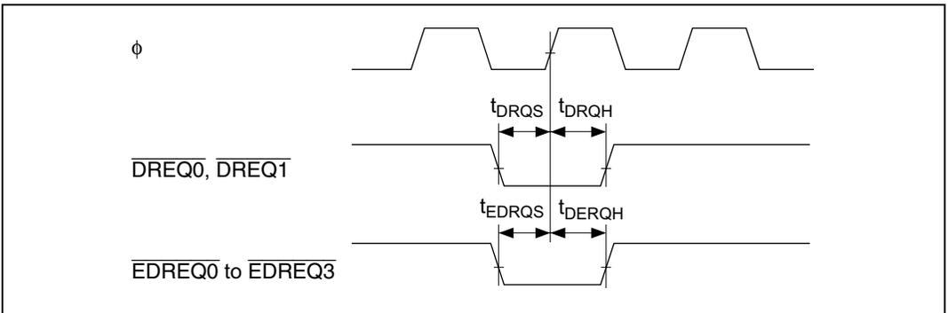
Figure 26.31 DMAC and EXDMAC  $\overline{DREQ}/\overline{EDREQ}$  Input Timing
