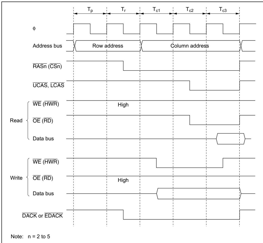
**Figure 6.42** Example of  $\overline{\text{DACK}}/\overline{\text{EDACK}}$  Output Timing when  $\text{DDS} = 0$  or  $\text{EDDS} = 0$
