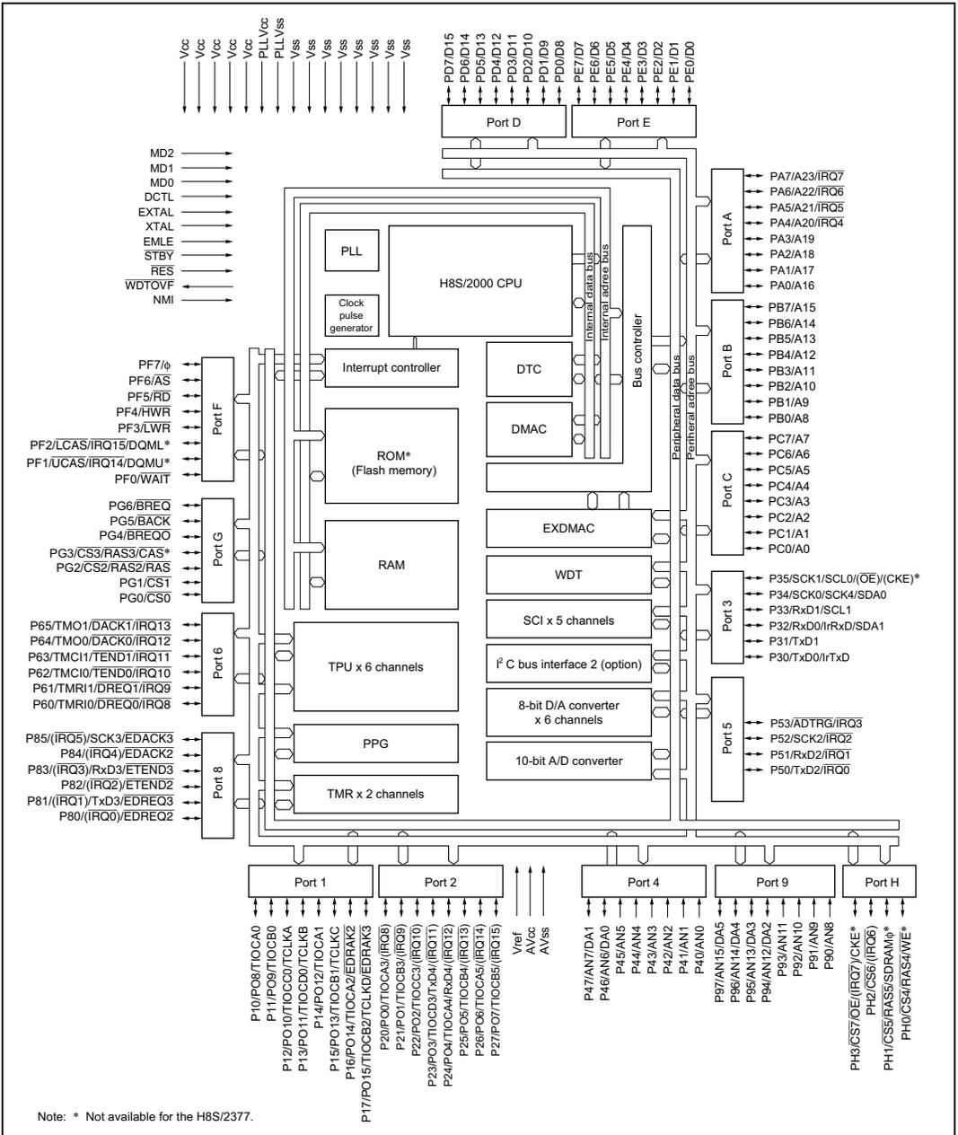
Figure 1.2 Internal Block Diagram for H8S/2377 and H8S/2377R
