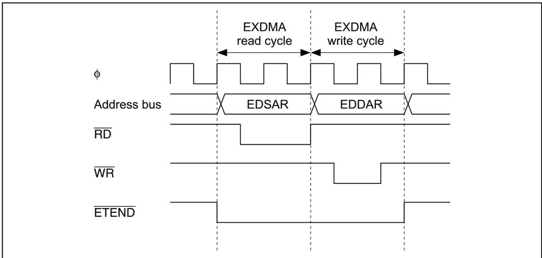
**Figure 8.2 Example of Timing in Dual Address Mode**
