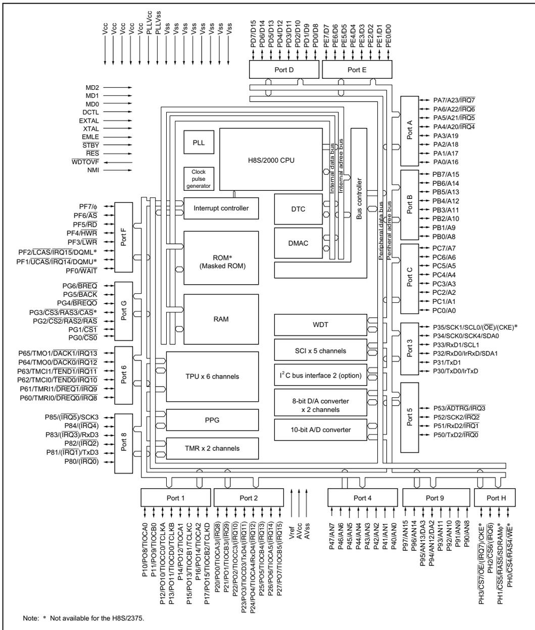
Figure 1.3 Internal Block Diagram for H8S/2375 and H8S/2375R
