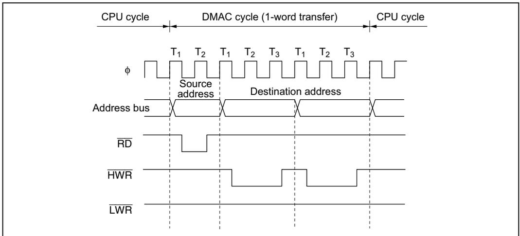
**Figure 7.17 Example of DMA Transfer Bus Timing**
