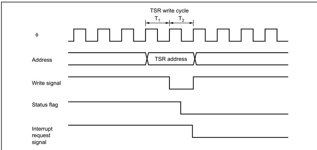
**Figure 11.42 Timing for Status Flag Clearing by CPU**
