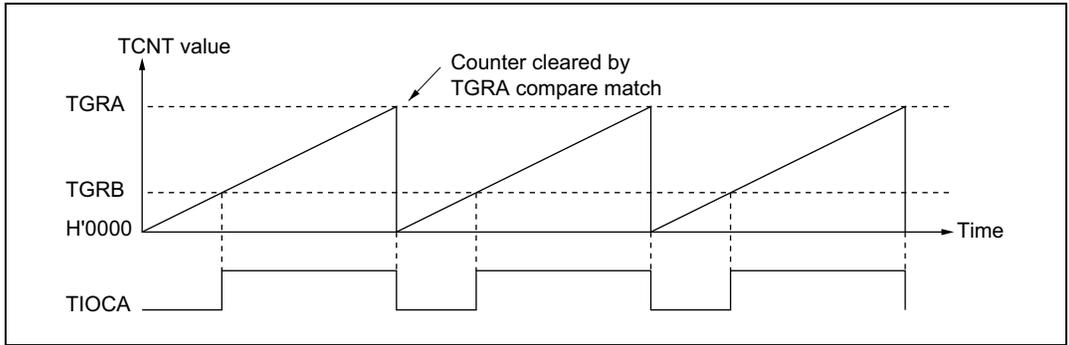
**Figure 11.21 Example of PWM Mode Operation (1)**
