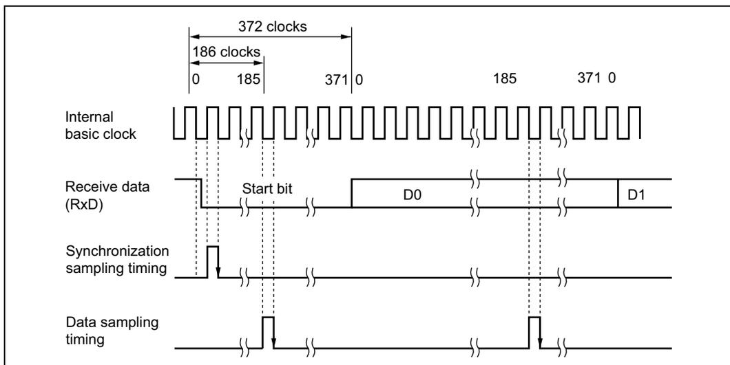
**Figure 15.25 Receive Data Sampling Timing in Smart Card Mode
