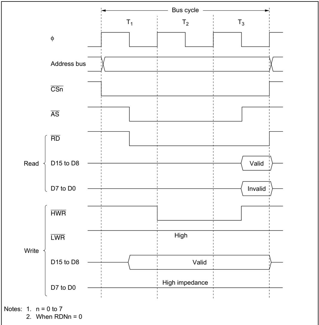
**Figure 6.15 Bus Timing for 16-Bit, 3-State Access Space
