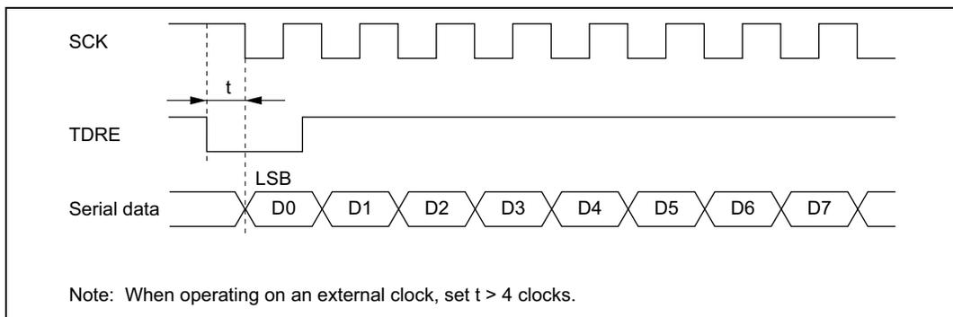
**Figure 15.35 Example of Synchronous Transmission Using DTC**
