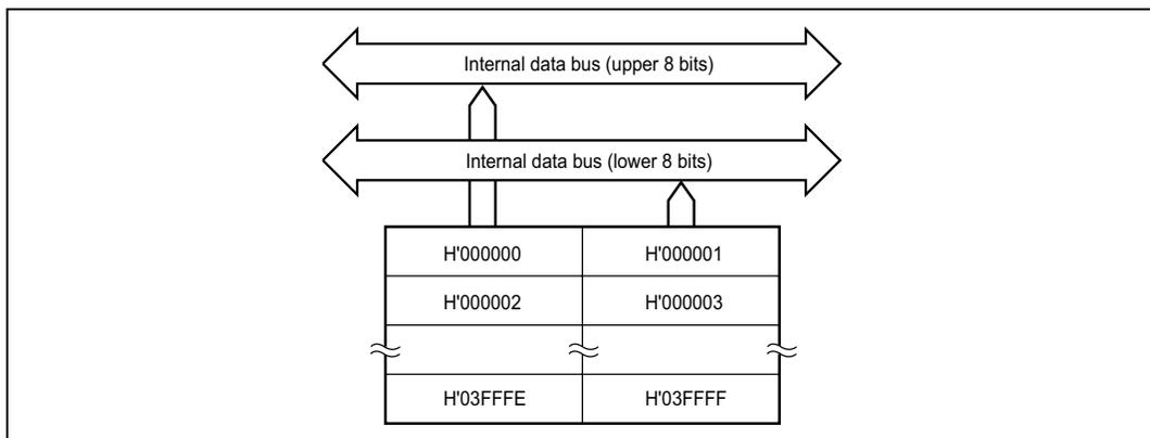
**Figure 22.1 Block Diagram of 256-kbyte Masked ROM (HD6432375)**
