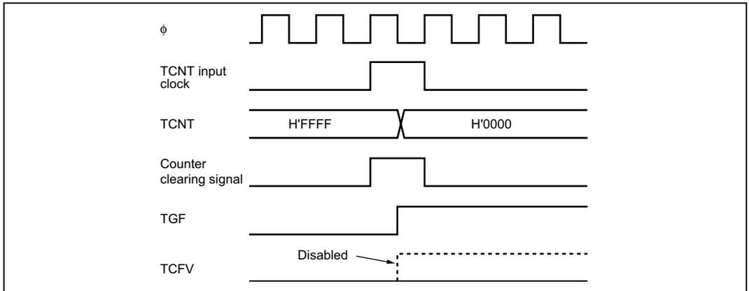
**Figure 11.52** Contention between Overflow and Counter Clearing
