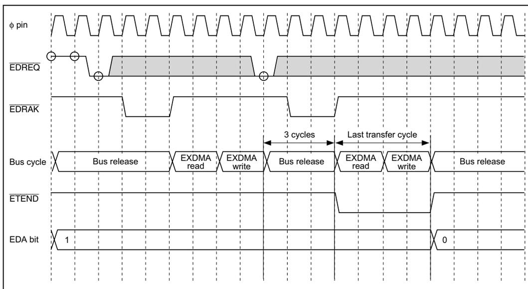
**Figure 8.35 External Request/Cycle Steal Mode/Normal Transfer Mode
