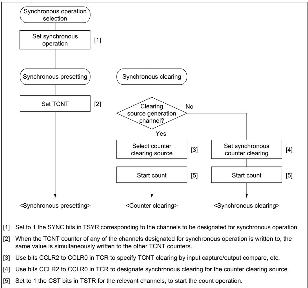
**Figure 11.10 Example of Synchronous Operation Setting Procedure**
