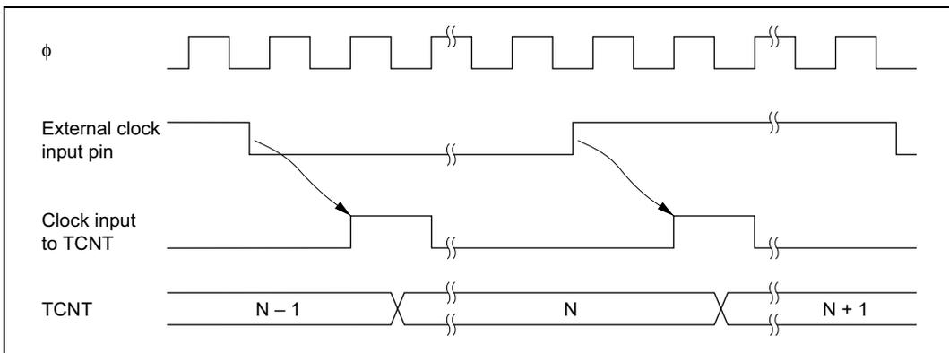
**Figure 13.4** Count Timing for External Clock Input
