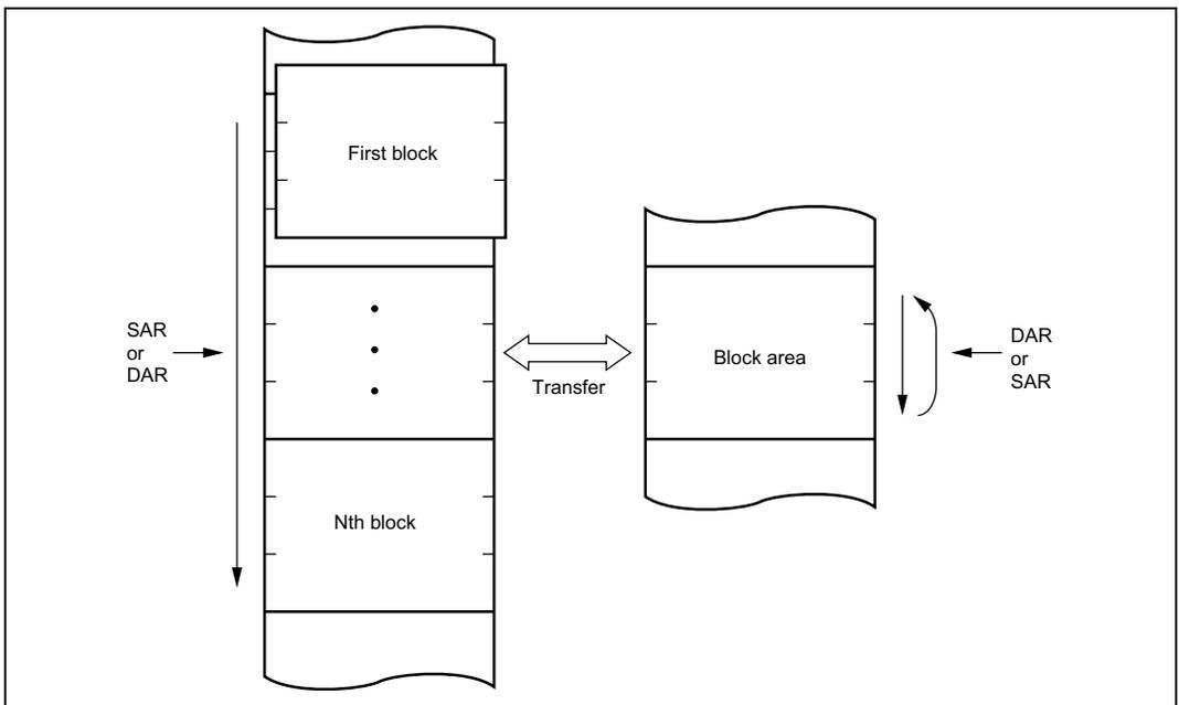
**Figure 9.8 Memory Mapping in Block Transfer Mode**
