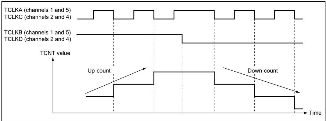
**Figure 11.26 Example of Phase Counting Mode 2 Operation**
