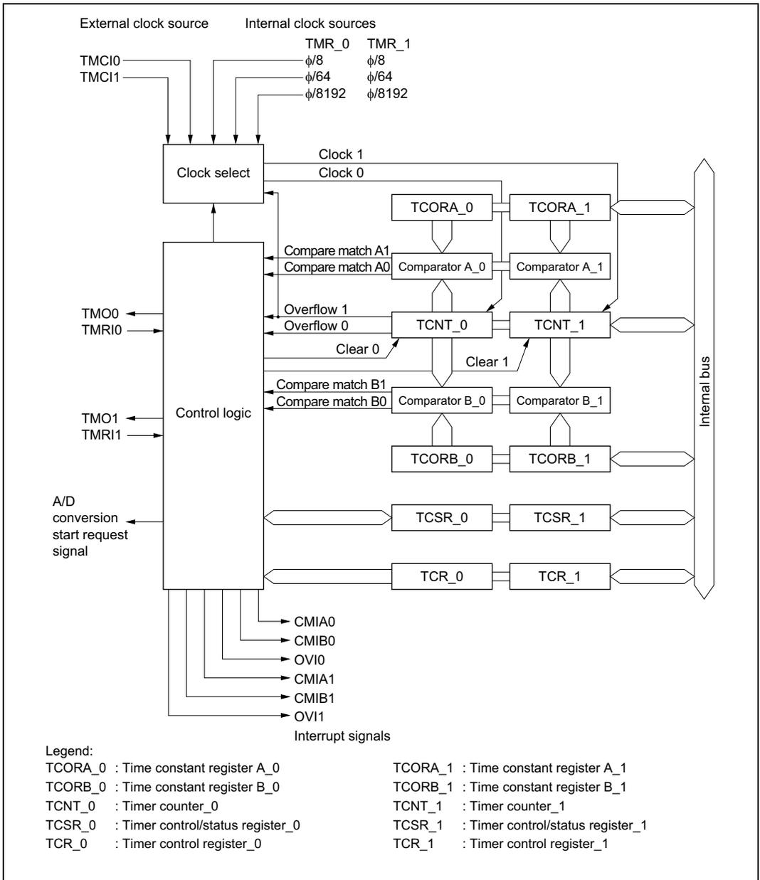
**Figure 13.1 Block Diagram of 8-Bit Timer Module**
