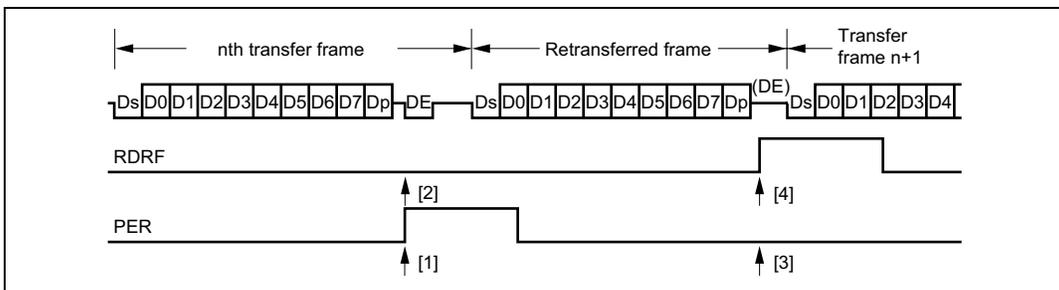
Figure 15.29 Retransfer Operation in SCI Receive Mode
