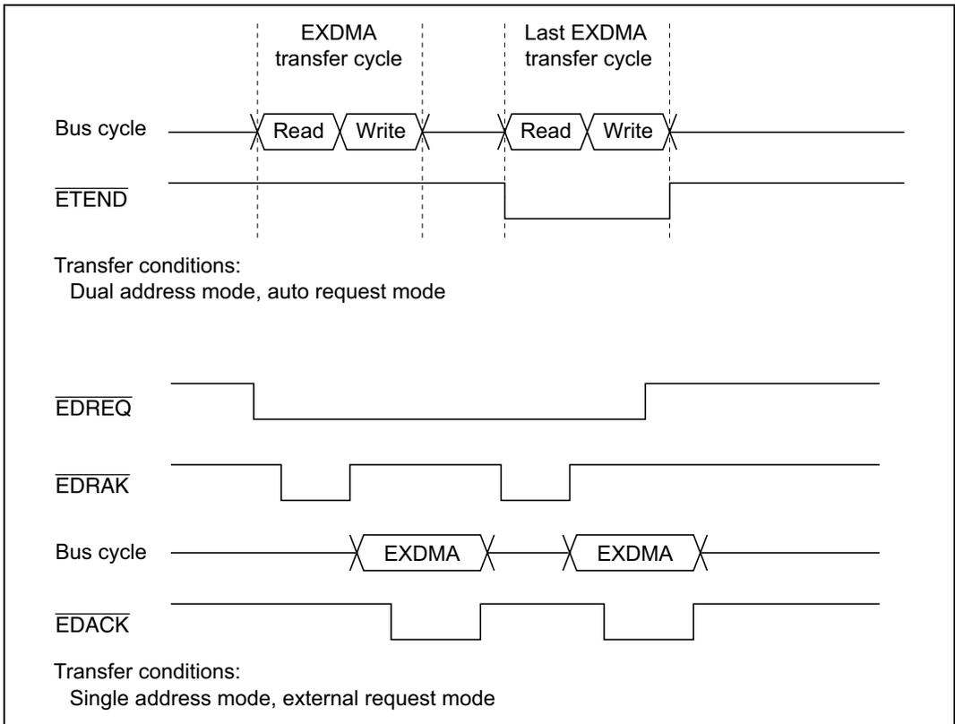
**Figure 8.7 Examples of Timing in Normal Transfer Mode**
