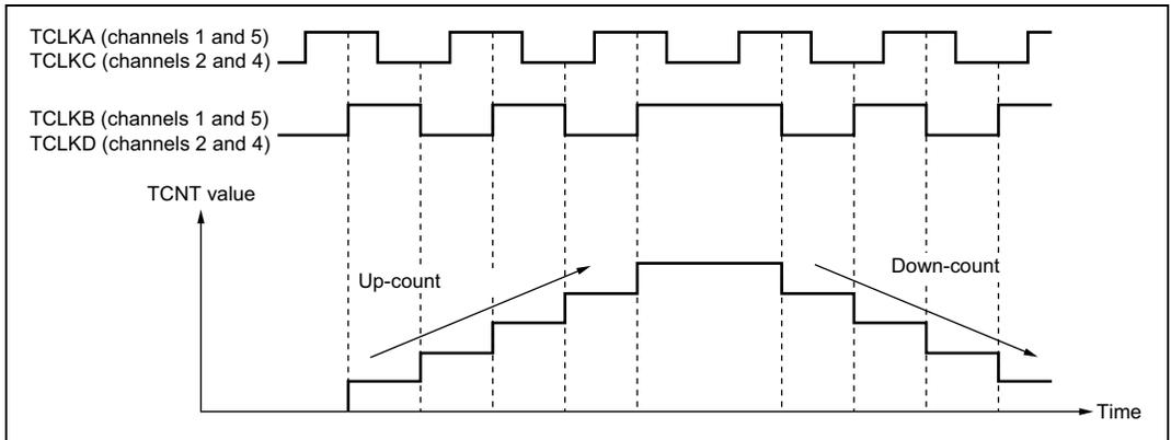
Figure 11.28 Example of Phase Counting Mode 4 Operation
