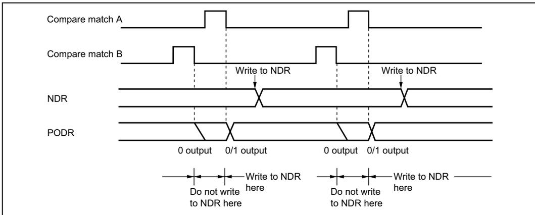
**Figure 12.7 Non-Overlapping Operation and NDR Write Timing**
