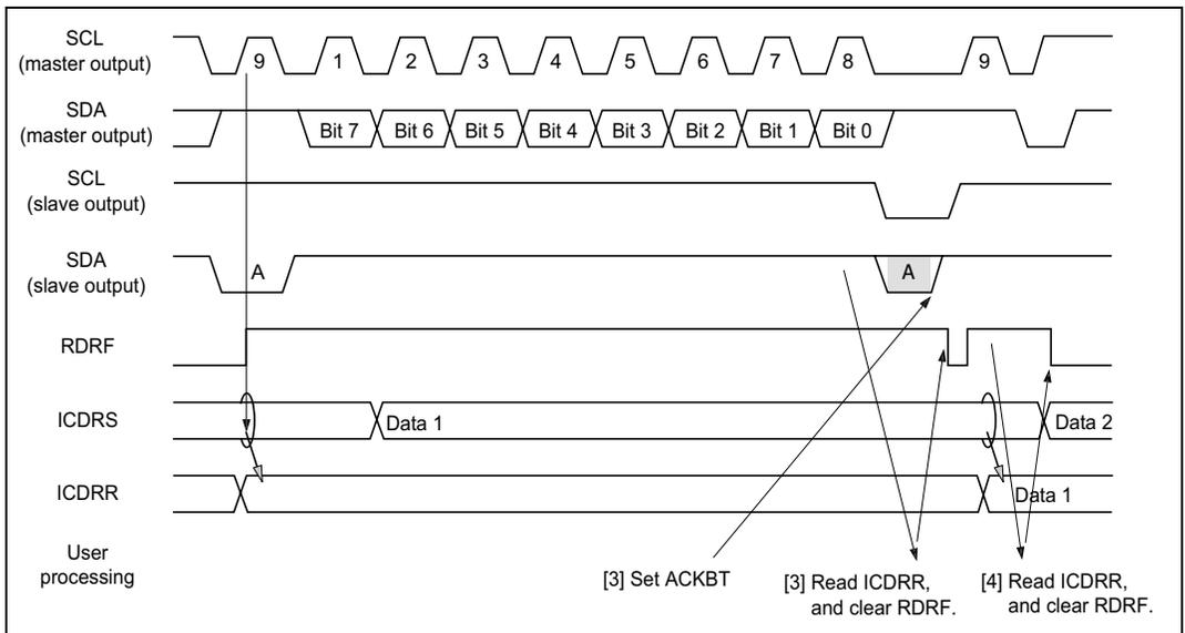
**Figure 16.12 Slave Receive Mode Operation Timing 2**
