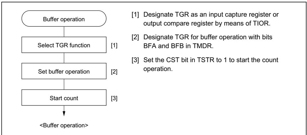
**Figure 11.14 Example of Buffer Operation Setting Procedure**
