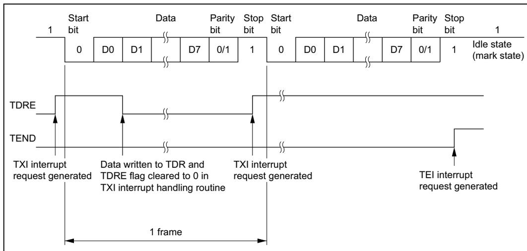
**Figure 15.6 Example of Operation in Transmission in Asynchronous Mode
