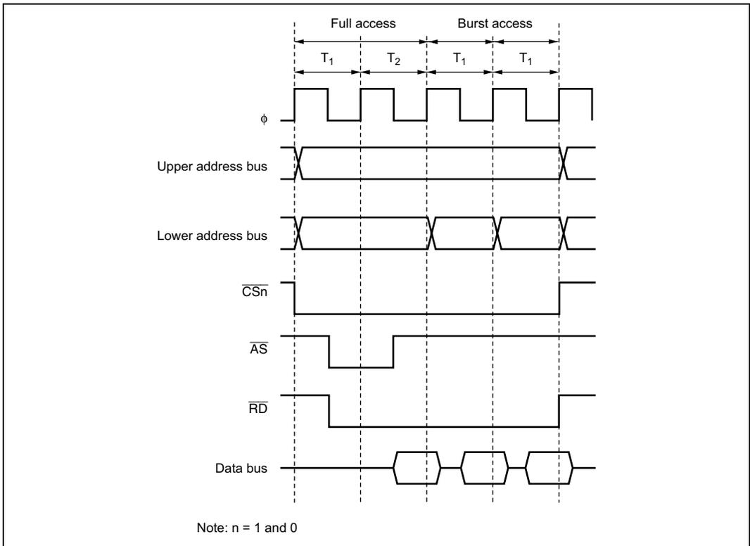
**Figure 6.64 Example of Burst ROM Access Timing
