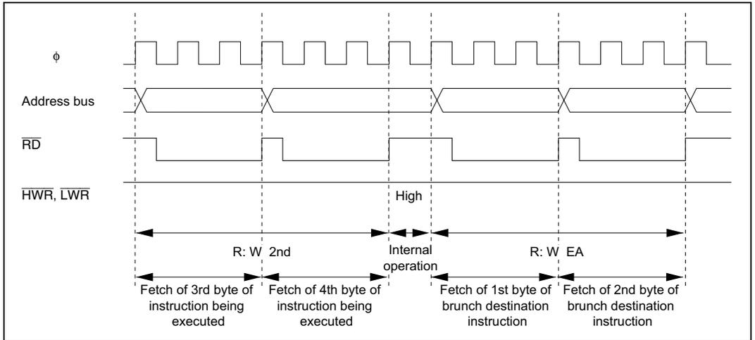
**Figure D.1 Timing of Address Bus,  $\overline{RD}$ ,  $\overline{HWR}$ , and  $\overline{LWR}$
