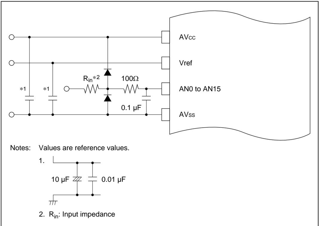
**Figure 17.7 Example of Analog Input Protection Circuit**
