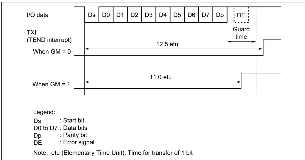
**Figure 15.27 TEND Flag Generation Timing in Transmission Operation**
