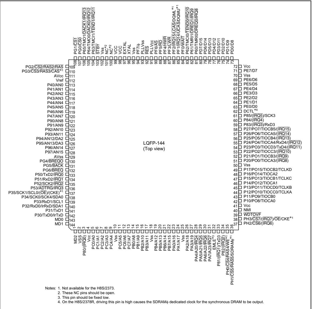
**Figure 1.8 Pin Arrangement for H8S/2373 and H8S/2373R**
