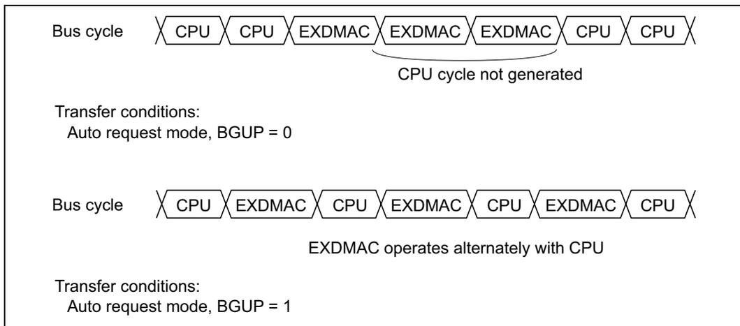
**Figure 8.6 Examples of Timing in Burst Mode**
