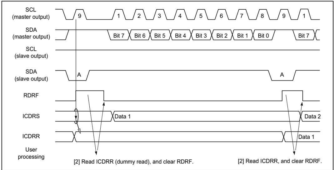
**Figure 16.11 Slave Receive Mode Operation Timing 1**
