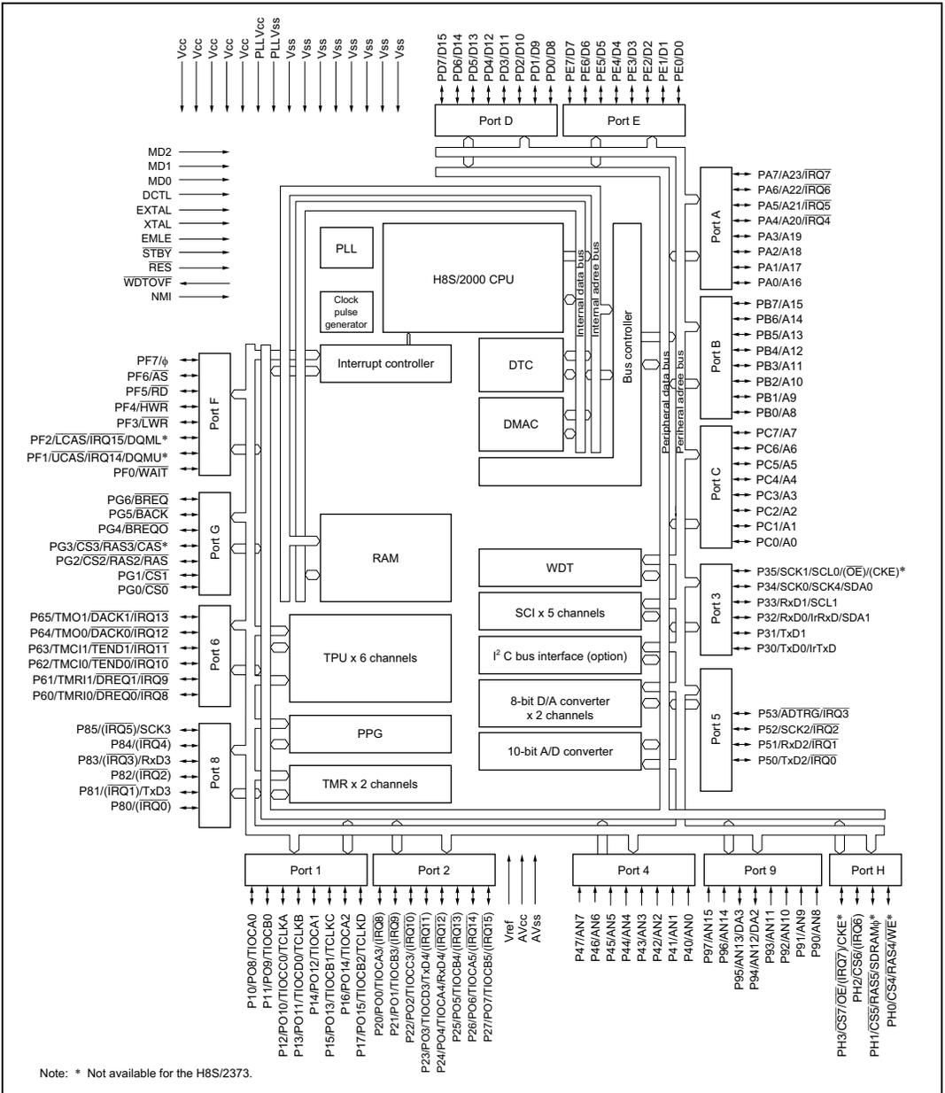
Figure 1.4 Internal Block Diagram for H8S/2373 and H8S/2373R
