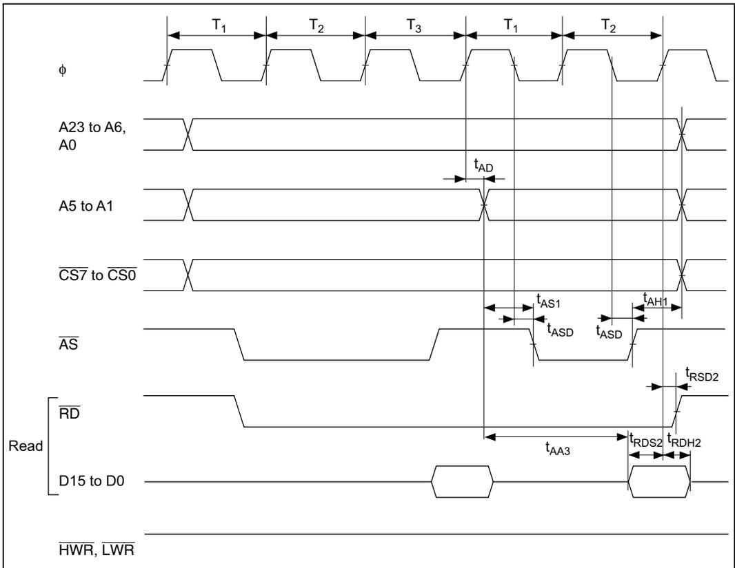
**Figure 26.13 Burst ROM Access Timing: Two-State Burst Access**
