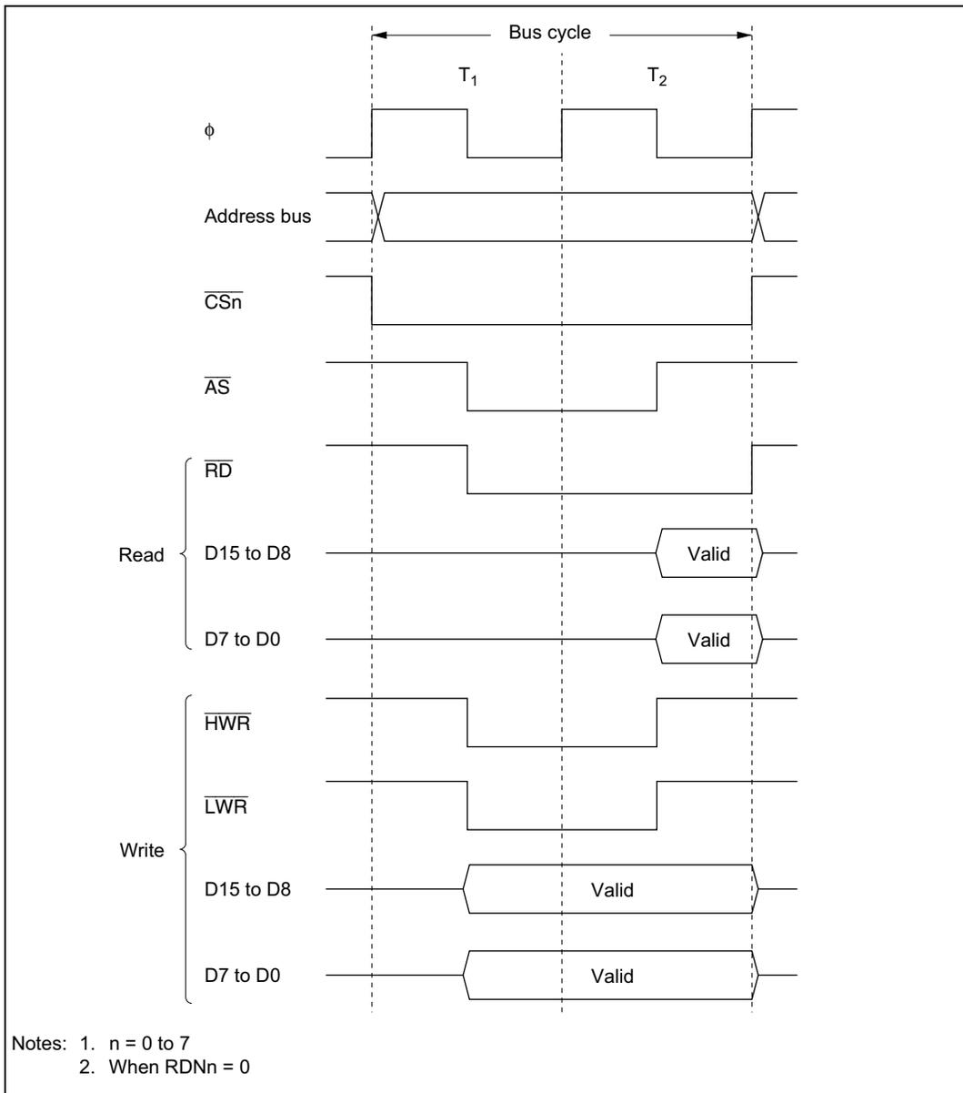
**Figure 6.14 Bus Timing for 16-Bit, 2-State Access Space
