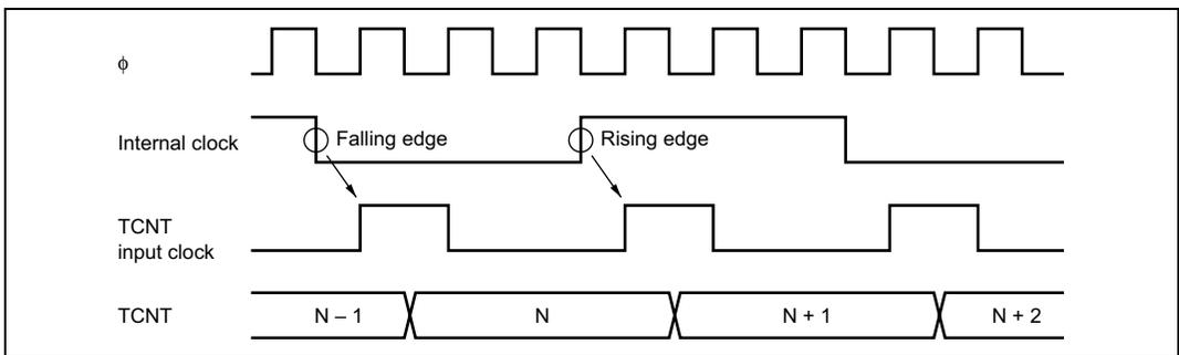
**Figure 11.30 Count Timing in Internal Clock Operation**
