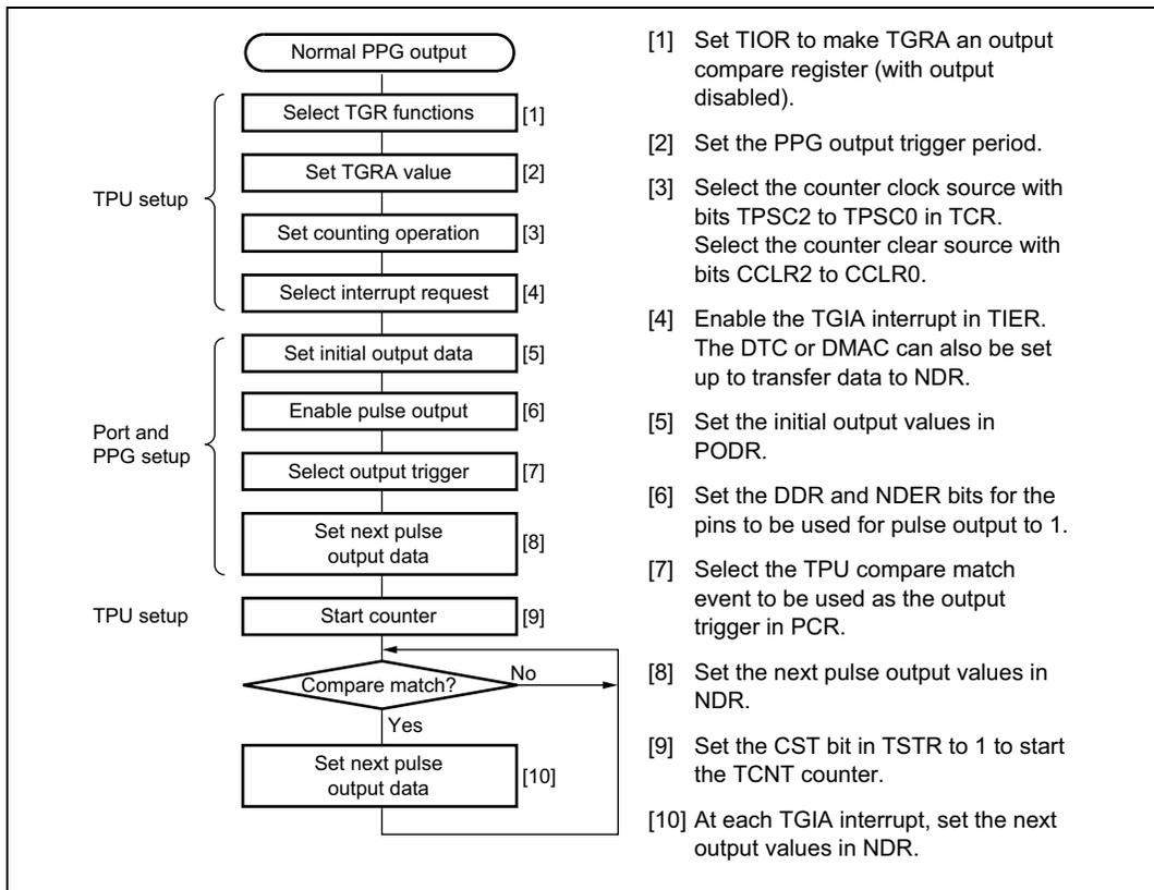
**Figure 12.4 Setup Procedure for Normal Pulse Output (Example)**
