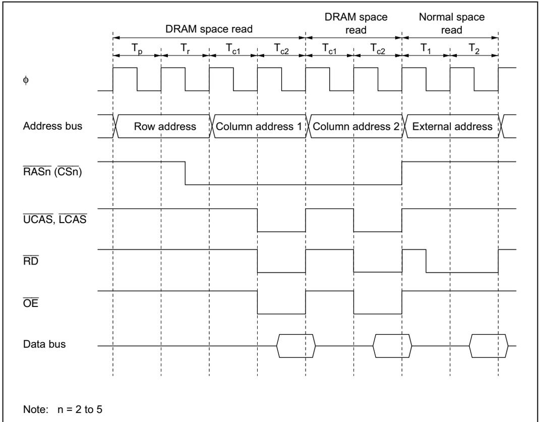
**Figure 6.33 Example of Operation Timing in RAS Up Mode**
