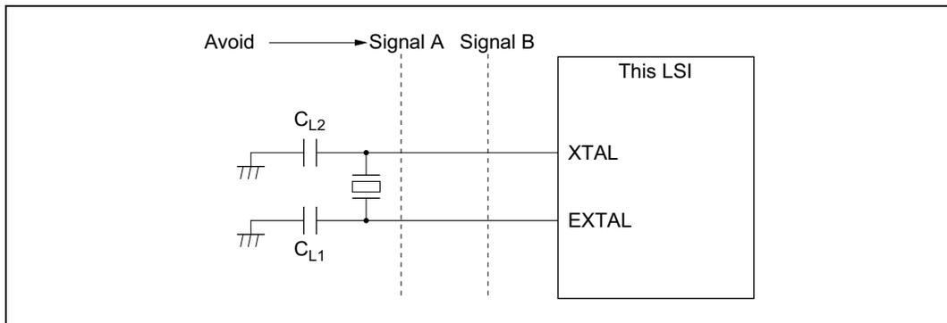
**Figure 23.6 Note on Board Design for Oscillation Circuit**
