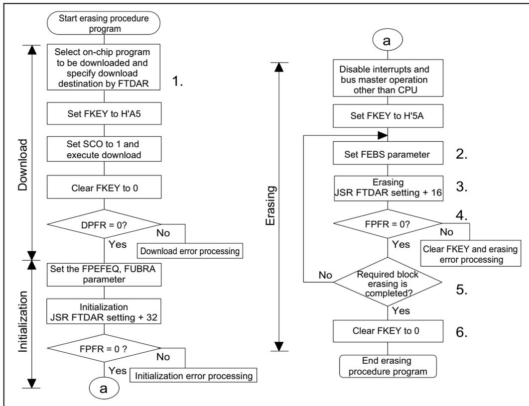
**Figure 21.12 Erasing Procedure**
