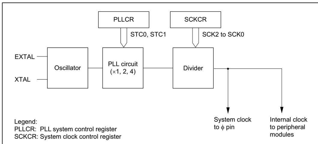
**Figure 23.1 Block Diagram of Clock Pulse Generator**
