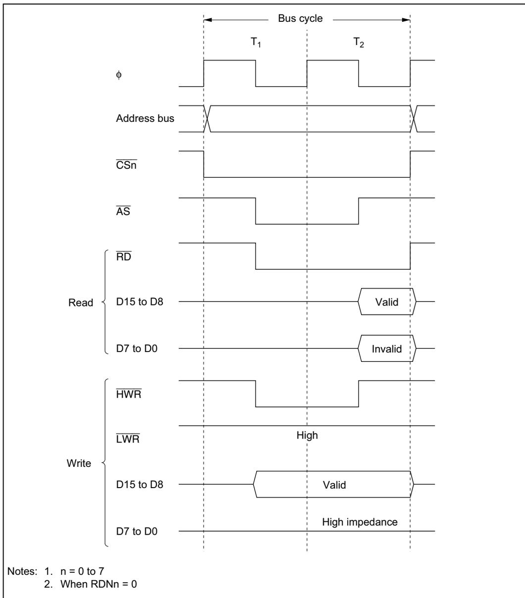
**Figure 6.12 Bus Timing for 16-Bit, 2-State Access Space
