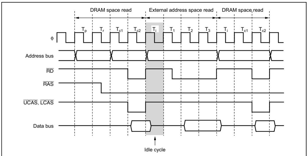
**Figure 6.76 Example of Idle Cycle Operation after DRAM Access
