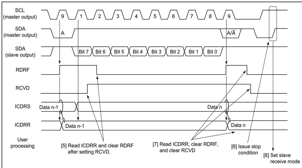
**Figure 16.8 Master Receive Mode Operation Timing 2**
