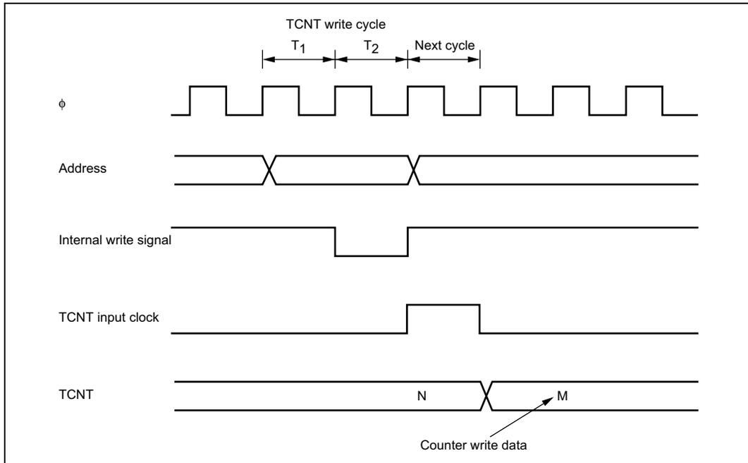
Figure 14.5 Contention between TCNT Write and Increment
