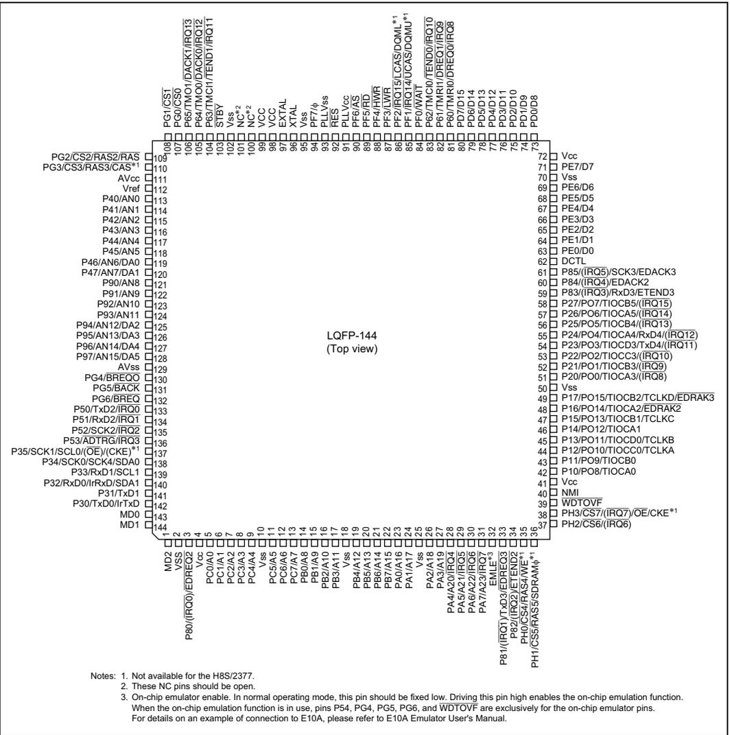
**Figure 1.6 Pin Arrangement for H8S/2377 and H8S/2377R**
