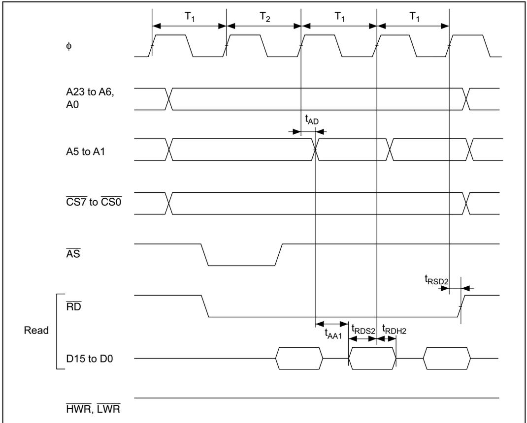
**Figure 26.12 Burst ROM Access Timing: One-State Burst Access**
