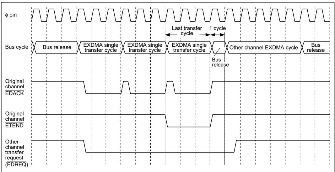
**Figure 8.34 Auto Request/Burst Mode/Normal Transfer Mode
