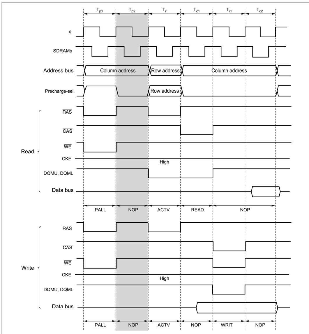
**Figure 6.47 Example of Timing with Two-State Precharge Cycle
