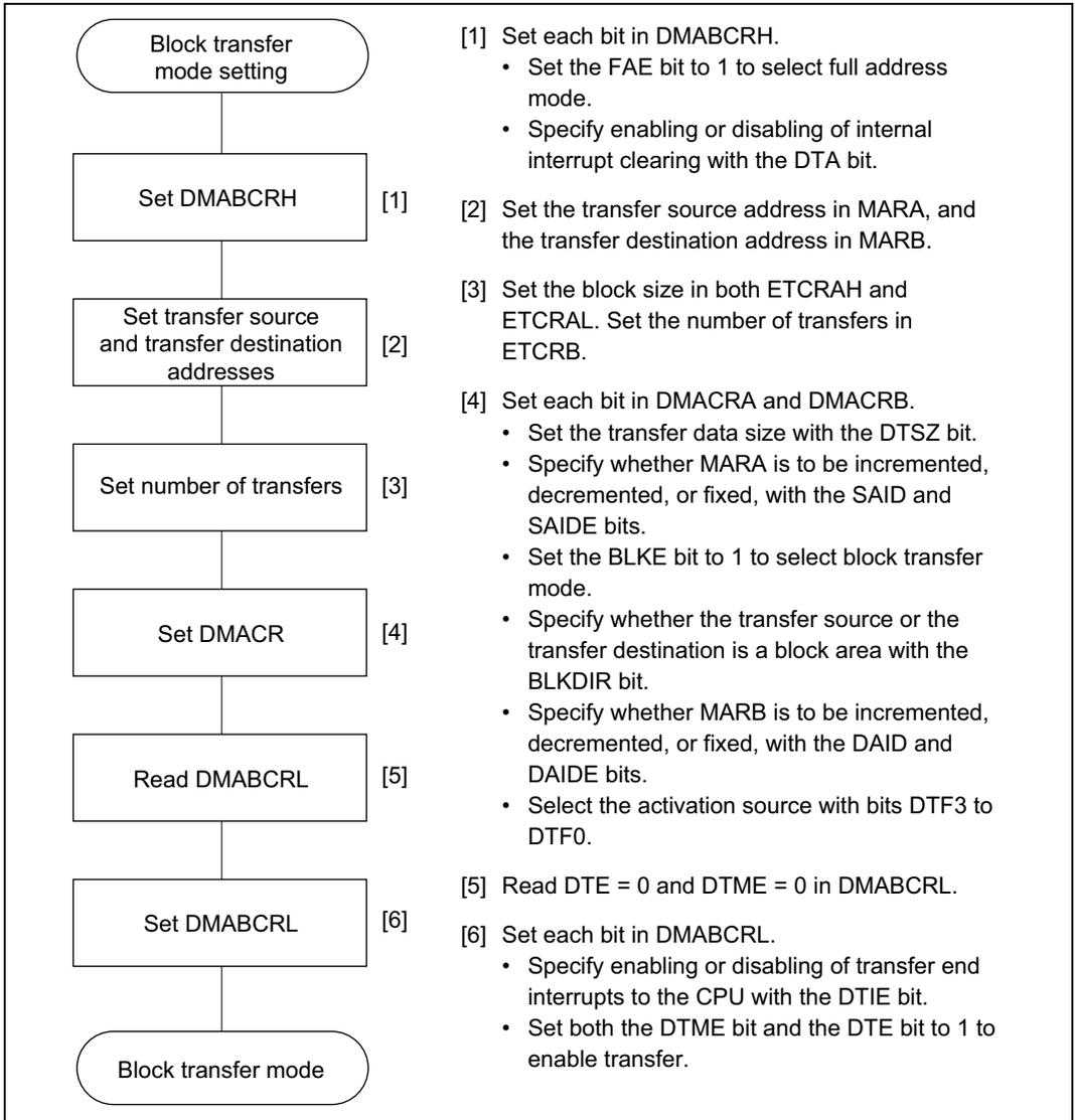
**Figure 7.16 Example of Block Transfer Mode Setting Procedure**
