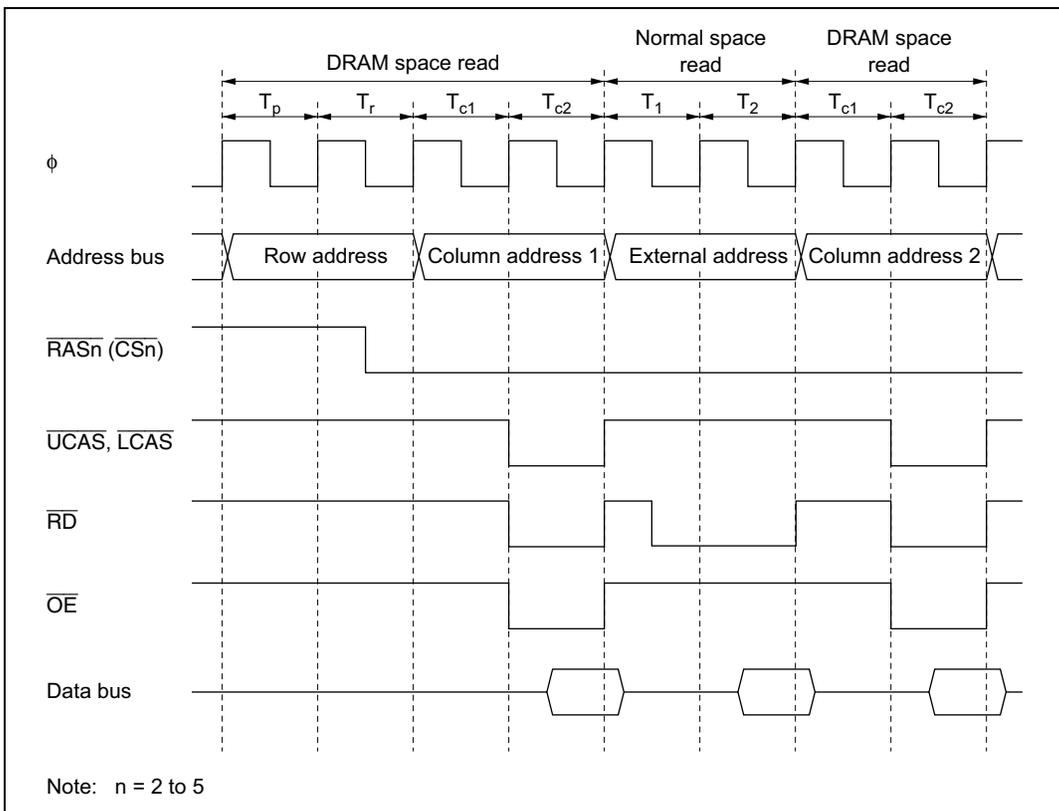
**Figure 6.32 Example of Operation Timing in RAS Down Mode
