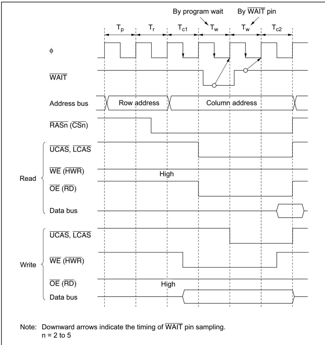
**Figure 6.26 Example of Wait State Insertion Timing
