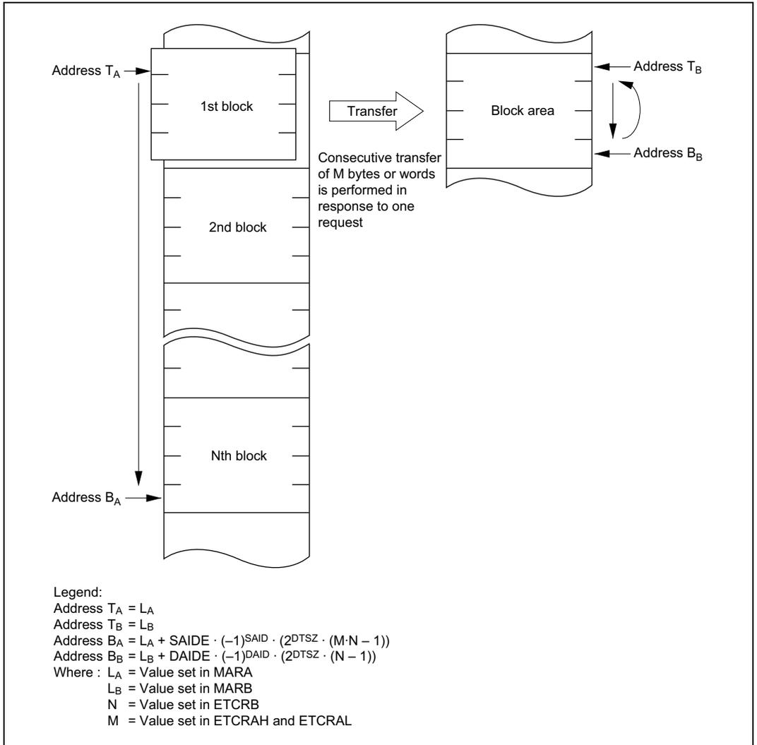
**Figure 7.13 Operation in Block Transfer Mode (BLKDIR = 0)**
