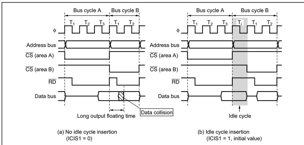
**Figure 6.65 Example of Idle Cycle Operation
