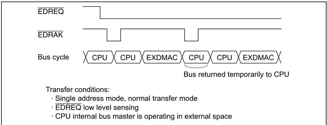
**Figure 8.5 Example of Timing in Cycle Steal Mode**
