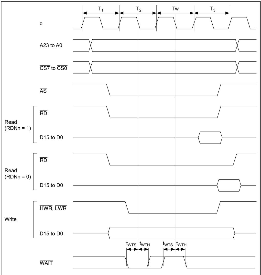
Figure 26.9 Basic Bus Timing: Three-State Access, One Wait
