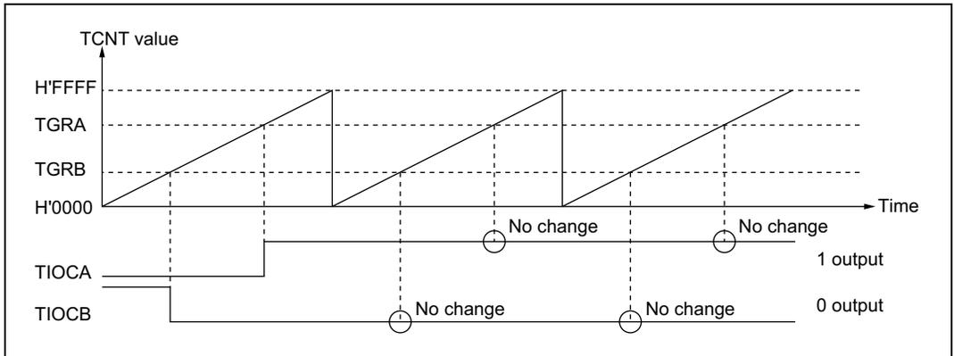
**Figure 11.6 Example of 0 Output/1 Output Operation**
