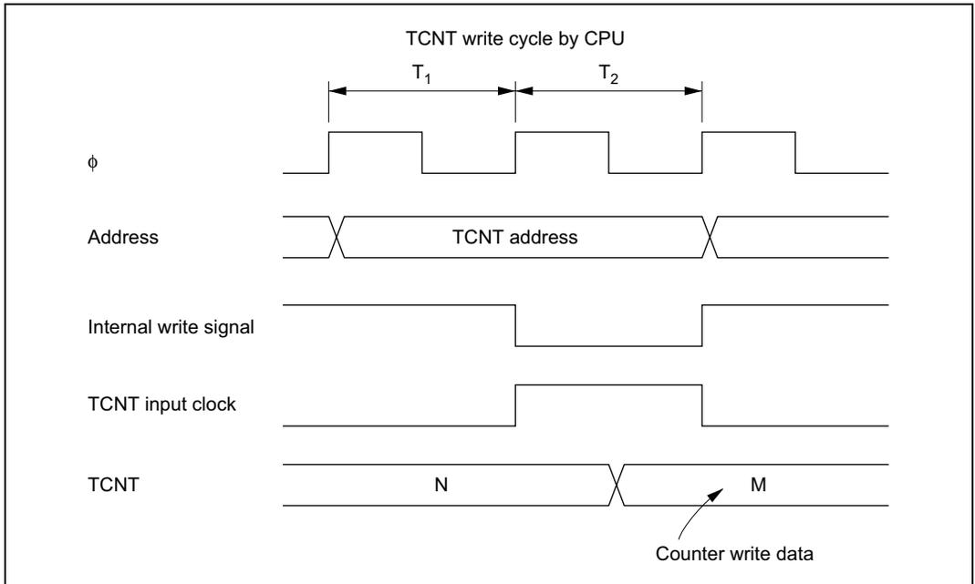
**Figure 13.11 Contention between TCNT Write and Increment**
