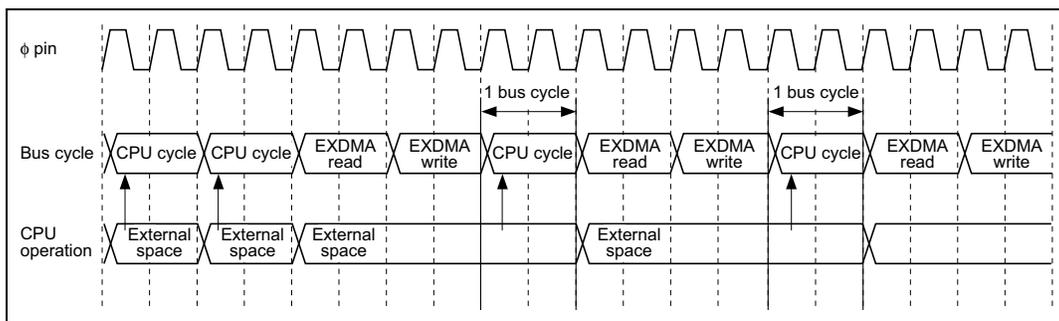
**Figure 8.32 Auto Request/Burst Mode/Normal Transfer Mode
