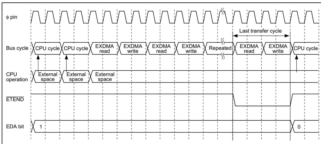
**Figure 8.31 Auto Request/Burst Mode/Normal Transfer Mode
