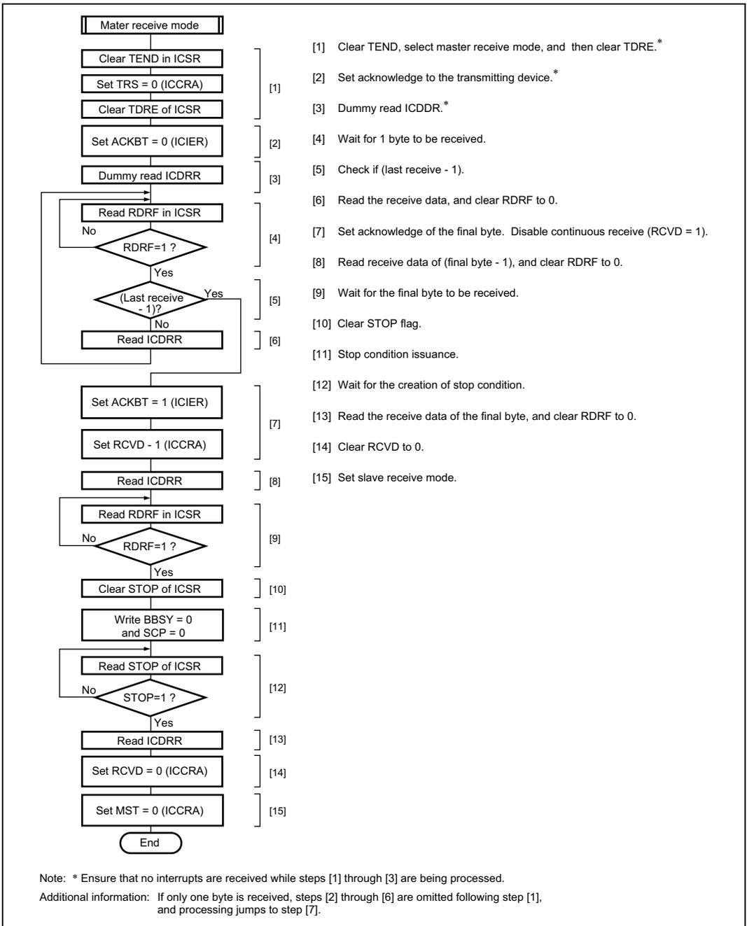
**Figure 16.15 Sample Flowchart for Master Receive Mode**
