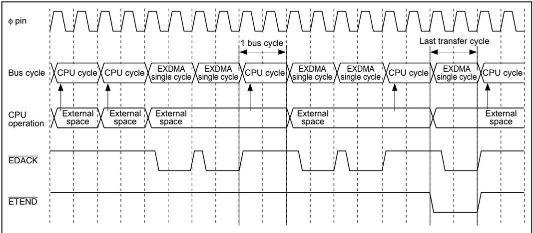
**Figure 8.33 Auto Request/Burst Mode/Normal Transfer Mode
