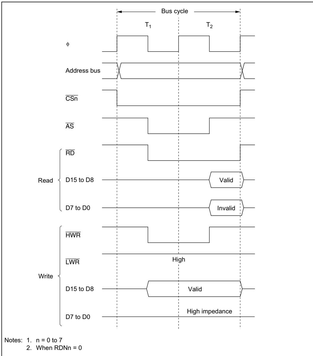
Figure 6.10 Bus Timing for 8-Bit, 2-State Access Space
