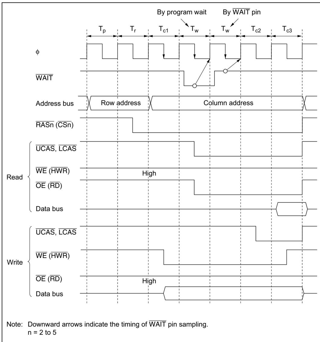
**Figure 6.27 Example of Wait State Insertion Timing
