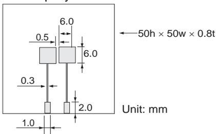
3. TURP is the structure which radiates heat to a substrate, please perform mounting to a substrate by reflow.
