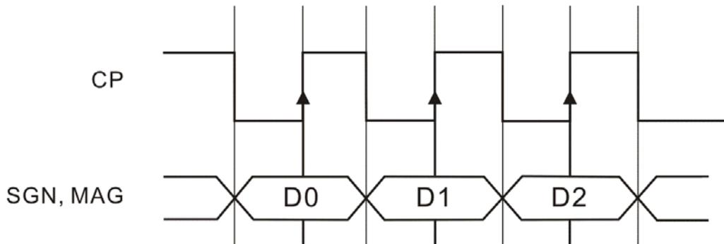
For the PT9120, the CP pin may be used as either clock input or output. With the on-chip reference crystal oscillator enabled, the CP pin becomes an output and delivers a CMOS-level signal with a nominal duty cycle of 50% at the same frequency as the reference crystal oscillator. By disabling the on-chip crystal oscillator (setting XEN to logic LOW), the CP pin becomes an input which accepts an external CMOS-level (TVSS to TVDD) clock signal with a duty cycle between 40% and 60%.
