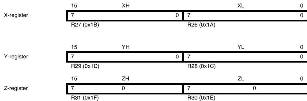
Figure 7-3. The X-, Y-, and Z-registers
