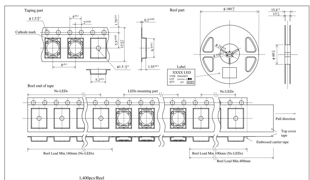
Taping is based on the **JIS C 0806**: Packaging of Electronic Components on Continuous Tapes.
