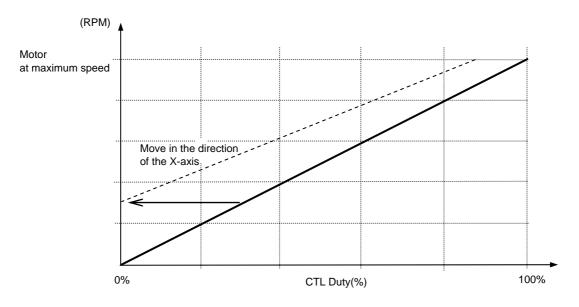
(Example) In the case where the characteristics change from ones with the origin point (0%, 0 rpm) to ones where the speed at a duty ratio of 30% becomes the speed at 0%:
