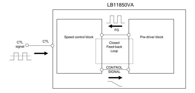
The operation inside the IC is as follows. Pulse signals are created from the edges of the FG signals as shown in the figure below, and a waveform with a pulse width which is determined by the CR time constants and which uses these edges as a reference is generated by a one-shot multivibrator.
