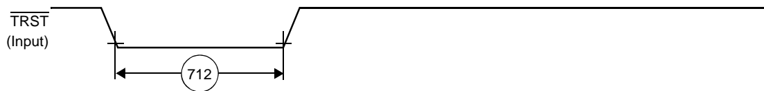
Figure 29. TRST Timing Diagram
