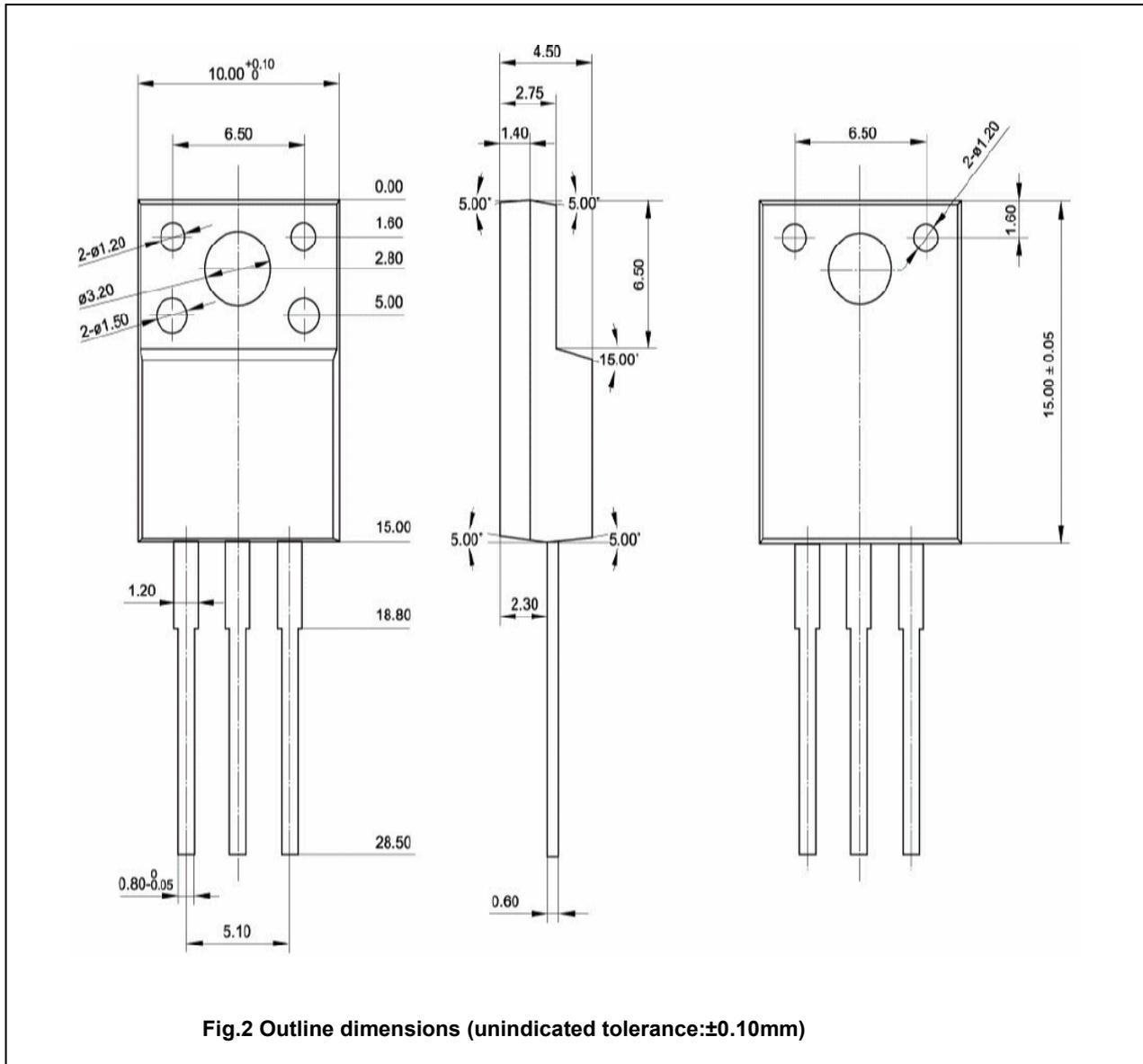
Fig.2 Outline dimensions (unindicated tolerance:±0.10mm)
