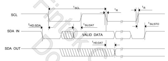
Serial Bus Timing Diagram
