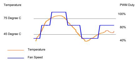
Below is a sample for Stage auto mode: Set temperature as 60°C, 40°C and Duty as 100%, 70%, 50%
