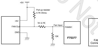
Fan with Tach Pull-Up to +5V, or Totern-Pole Output and Register Attenuator
