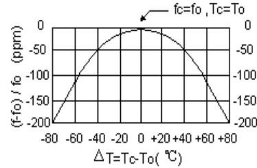
The curve shown above accounts for resonator contribution only and does not include oscillator temperature characteristics.
