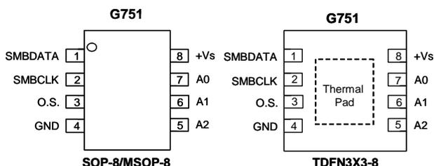
Note: Recommend connecting the Thermal Pad to the GND or let it keep floating.
