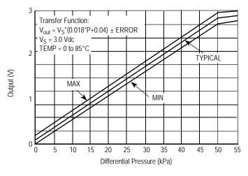
Figure 2. Output versus Pressure Differential
