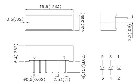
1.All dimensions are in millimeters (inches), Tolerance is  $\pm 0.25(0.01")$  unless otherwise noted. 2.Specifications are subject to change without notice.
